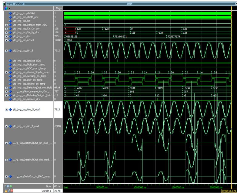
Figure 10. Total operation simulation result of the FPGA signal processing algorithm.
