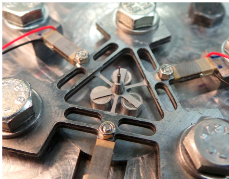
Figure 2. Assembled probing system, with stylus length 5.6 mm and 300 \mu\text{m} diameter ruby tip.
