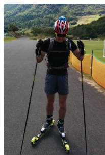
Figure 5. Locations of inertial sensors on wrists and in front of the bindings of roller skis. A video camera is located on the left shoulder strap.
