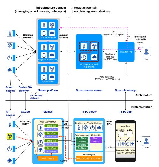
Figure 1. System architecture and implementation for IoT-based smart services.
