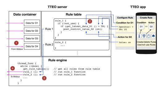
Figure 4. TTEO service server operation: create rules and run its rule engine.
