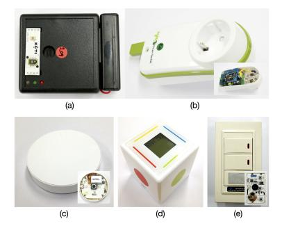
**Figure 2.** Prototype IoT devices: (**a**) multi-functional sensor for measuring temperature, humidity, illumination, and occupancy; (**b**) smart plug; (**c**) wireless switch; (**d**) smart dice; and (**e**) wall light switch.
