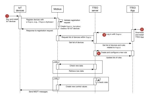
Figure 5. A sequence diagram for operating procedure of TTEO service.
