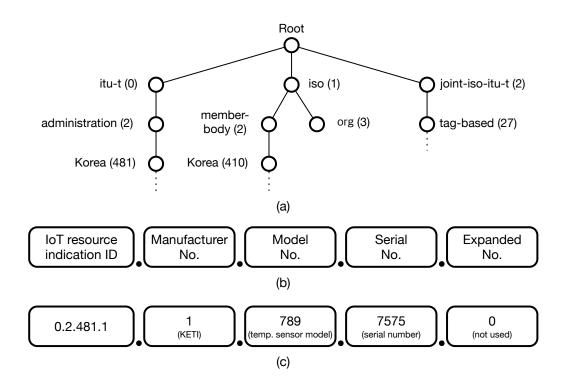
**Figure 8.** The OID-based IoT resource identification structure: (**a**) the OID hierarchy, (**b**) the proposed ID structure for IoT devices, (**c**) an OID example of the temperature sensor whose manufacturer is KETI, model number 789, and serial number 7575, provided the root for IoT resource indication in Korea is 0.2.481.1.
