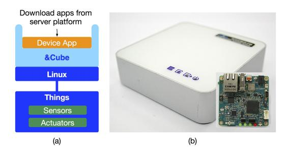
**Figure 3.** The &Cube and IoT gateway: (**a**) architecture of our device software platform (&Cube) and (**b**) the IoT gateway developed (IoTG100) on which the &Cube is running.
