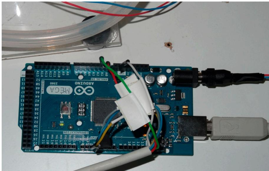
Figure 11. Arduino MEGA connected under laboratory tests.
