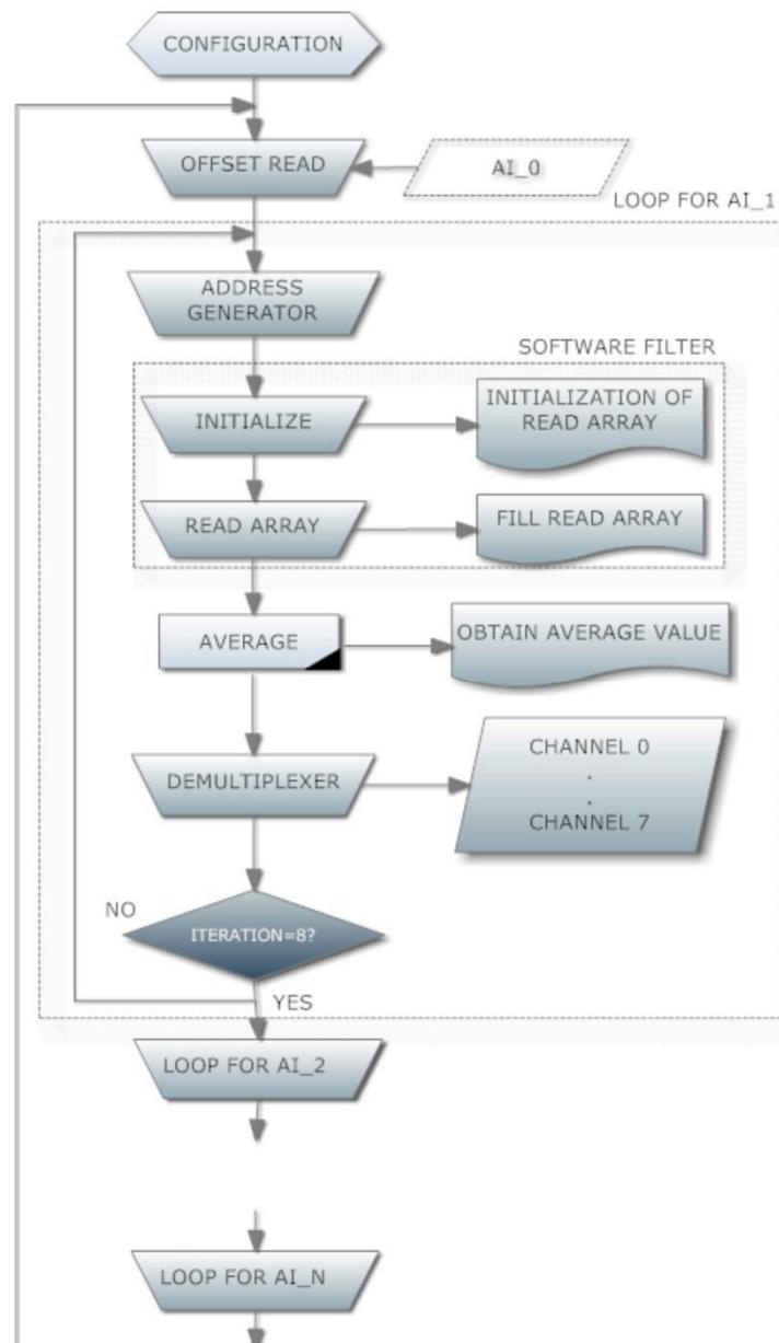
**Figure 6.** Flowchart of the NI LabVIEW program.
