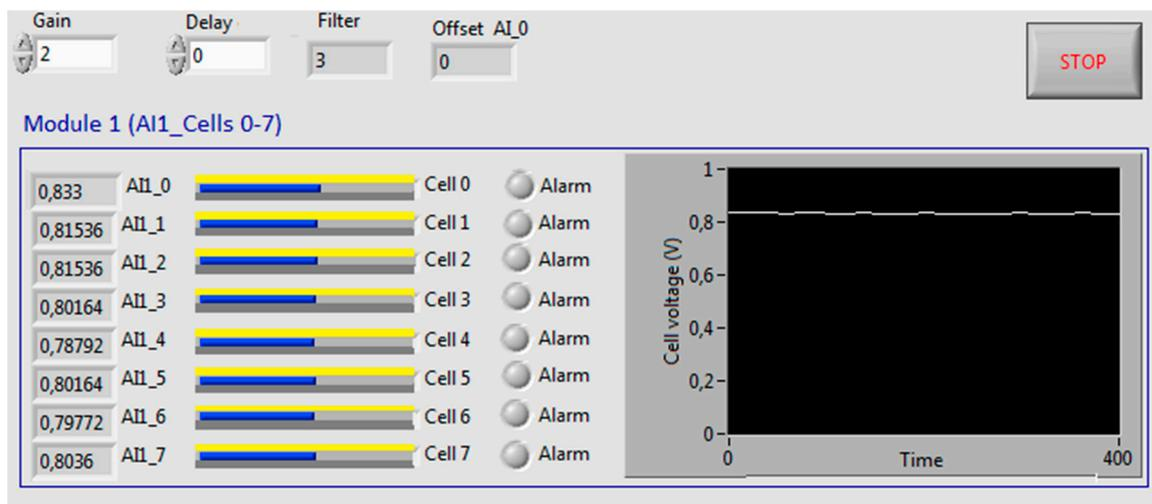
Figure 12. GUI during open circuit test.
