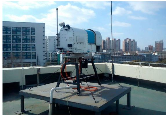
**Figure 1.** The water vapor radiometer used for data collection on the roof of Cehui building on the Tongji campus (Shanghai, China).
