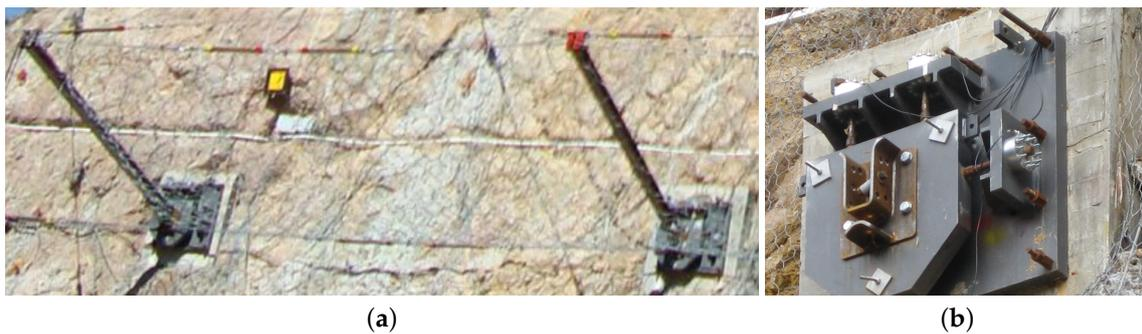
**Figure 7.** Post base measurement system (a) with installed posts at a test site and (b) in detail showing three pressure sensors orthogonal to the rock face and three two-way sensor installations parallel to the rock face (source: Igor Paramassi S.p.a.).
