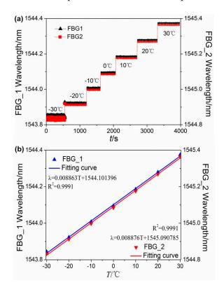
**Figure 4.** Temperature responses. (**a**) Wavelength shift as a function of temperature; (**b**) relationship between temperature variation and wavelength.
