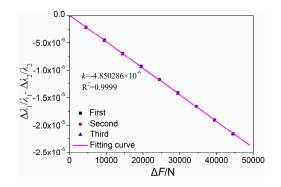
Figure 8. Relationship between load variation and relative wavelength shift difference.
