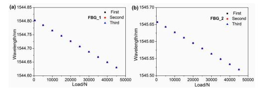
Figure 7. Relationship between load variation and wavelength of (a) FBG\_1 and (b) FBG\_2.
