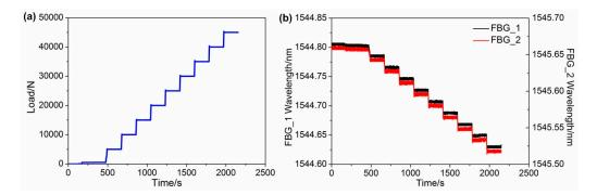
**Figure 6.** (a) Load variation of the universal testing machine; (b) real-time load response of the two FBGs.
