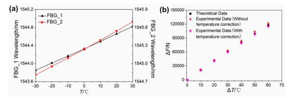
**Figure 10.** (a) Relationship between the central wavelength and the temperature variation; (b) comparison between measured and theoretical values.
