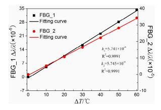
Figure 5. Relationship between the relative shifts of the central wavelength and the temperature variation.
