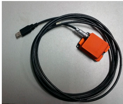
Figure 11. The motion capture system based on inertial technology.
