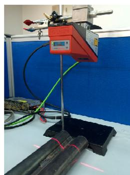
**Figure 12.** Measurement of cylindrical objects welded together.
