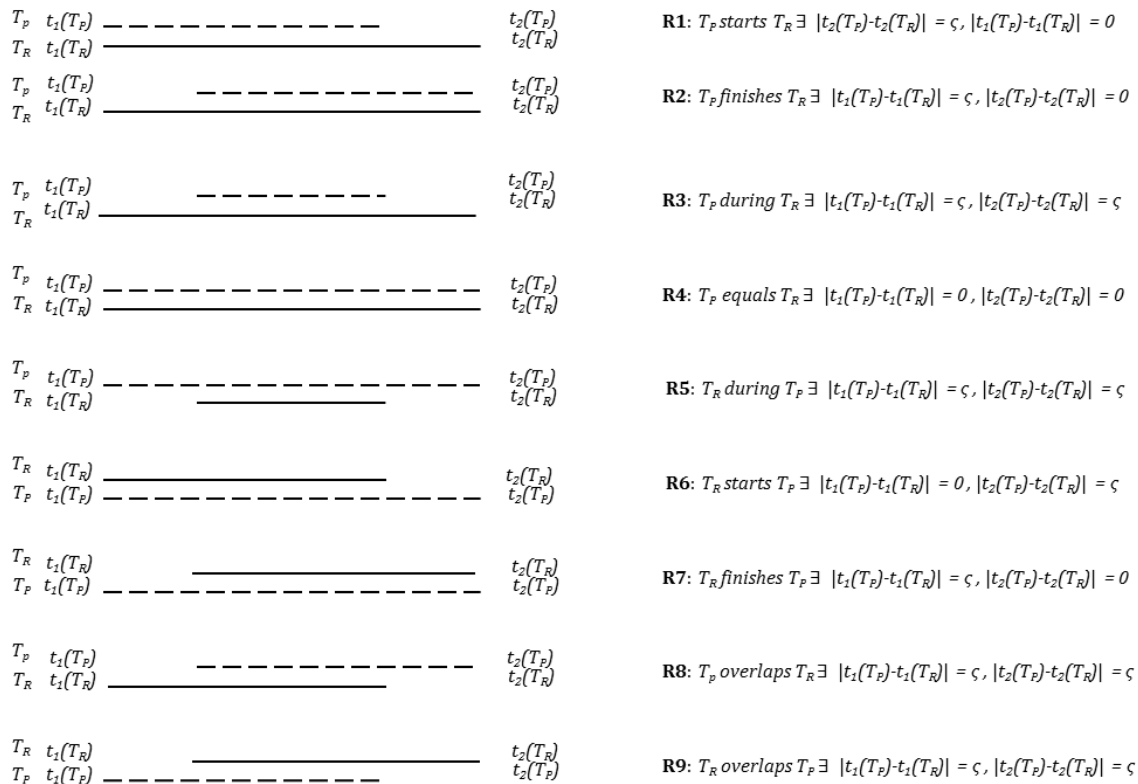
Figure 1. Trip uncertain temporal relationships between a reported trip ( T_R ) and predicted trip ( T_P ) based on Allen's temporal calculus. In this figure t_1 and t_2 are the start time and end time of a given trip respectively.
