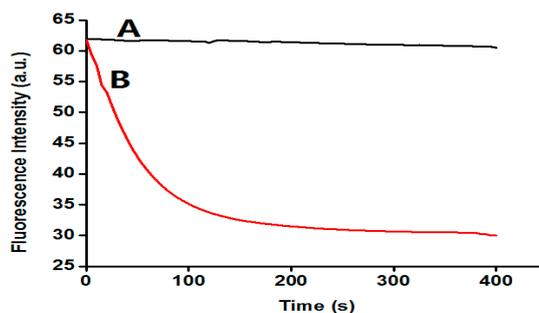
**Figure 2.** Fluorescence spectra of this sensing system in the absence (A) and presence (B) of 500 nM  $\text{Hg}^{2+}$  ions (50 nM DNA probe, 50  $\mu\text{M}$  dNTP, 20 U/mL KF polymerase).
