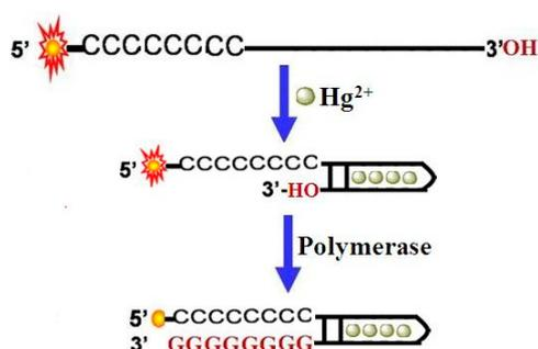
**Figure 1.** Schematic diagram of detection of  $\text{Hg}^{2+}$  based on polymerase-aided photoinduced electron transfer strategy.
