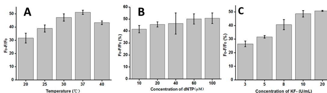
**Figure 3.** Optimization of the reaction conditions: (A) temperature (50 nM DNA probe, 50 μM dNTP, 20 U/mL KF polymerase); (B) concentration of dNTP (50 nM DNA probe and 20 U/mL KF polymerase); (C) concentration of KF polymerase (50 nM DNA probe and 60 μM dNTP). Error bars show the standard deviation of three experiments.
