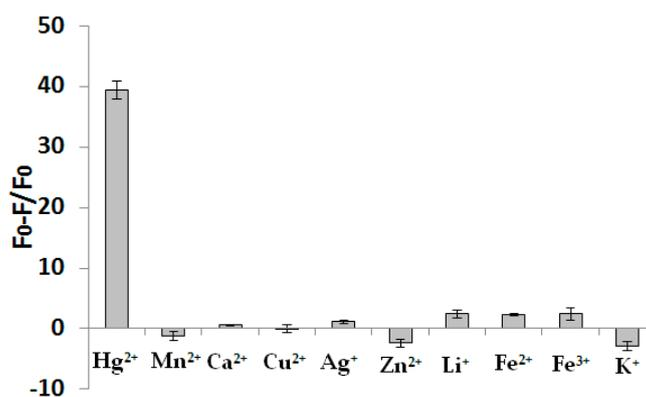
**Figure 5.** Selectivity of the analysis of Hg<sup>2+</sup> by our method. The concentration of Hg<sup>2+</sup> was 100 nM, and the concentrations of Mn<sup>2+</sup>, Ag<sup>+</sup>, Ca<sup>2+</sup>, Cu<sup>2+</sup>, Zn<sup>2+</sup>, Li<sup>+</sup>, Fe<sup>2+</sup> and Fe<sup>3+</sup> were kept at 2 μM and the concentration of K<sup>+</sup> was 20 mM (50 nM DNA probe, 60 μM dNTP, 20 U/mL KF polymerase). Error bars show the standard deviation of three experiments.
