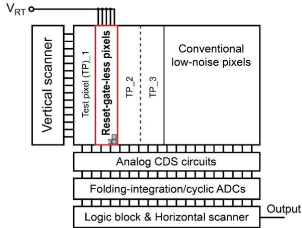
**Figure 11.** Block diagram of the experimental CIS chip.
