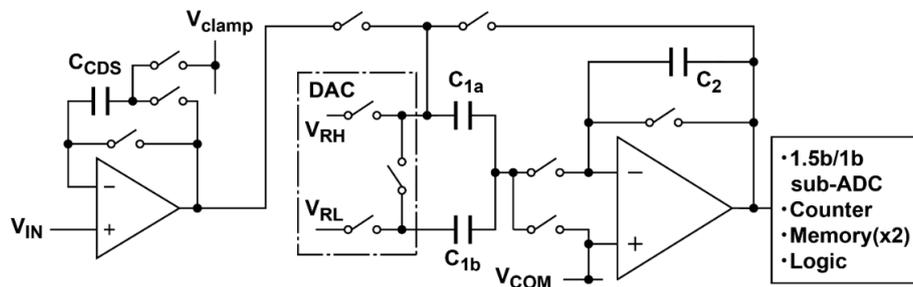
Figure 12. Column analog CDS and ADC circuits.
