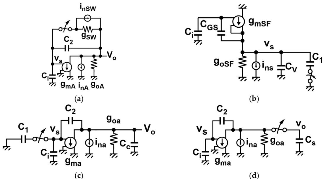
**Figure 7.** Equivalent circuits for noise calculation at four phases of Figure 3. (a) Integrator resetting (Figure 3a); (b) input signal sampling (Figure 3b); (c) signal charge transfer (Figure 3c); and (d) integrator output sampling for ADC (Figure 3d).
