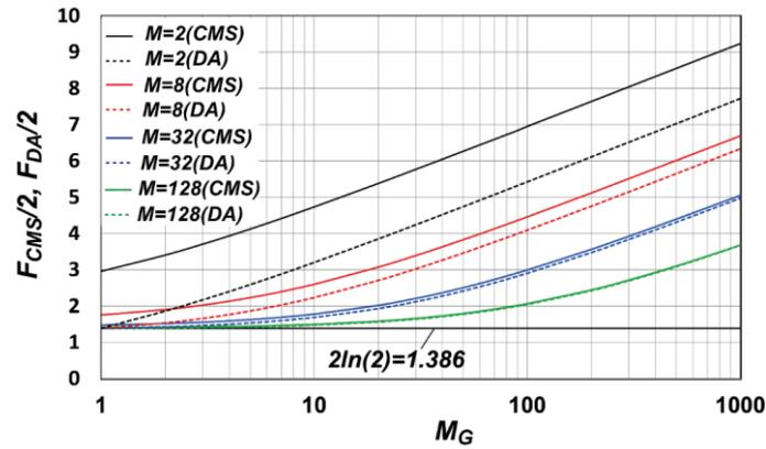
**Figure 8.** Noise reduction factor of the CMS,  $F_{CMS}$ , and differential averager,  $F_{DA}$ , as a function of  $M_G$  and  $M$ .
