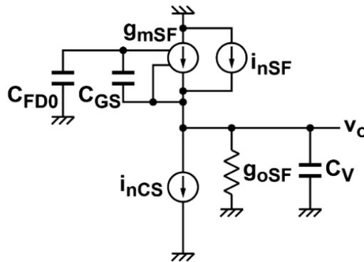
**Figure 5.** Equivalent circuit of the pixel source follower for noise analysis.
