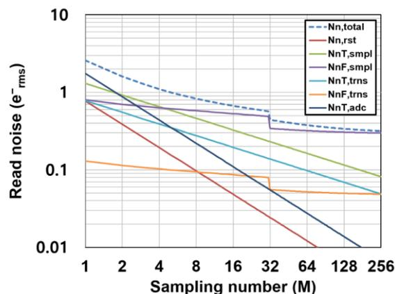
**Figure 14.** Noise components as a function of the sampling number in the folding-integration ADC.
