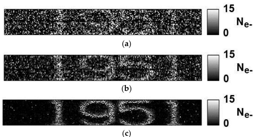
Figure 16. Low-light-level images with three different CMS gains ( $M = 2, 16$ , and  $128$ ). (a)  $M = 2$ , noise (median):  $2.4 e^-_{rms}$ ; (b)  $M = 16$ , noise (median):  $1.1 e^-_{rms}$ ; and (c)  $M = 128$ , noise (median):  $0.29 e^-_{rms}$ .
