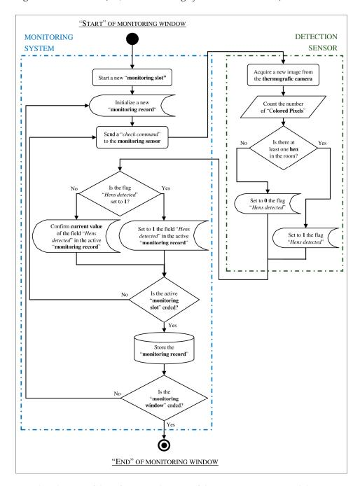
Figure 2. Flow diagram of the software applications of the monitoring system and detection sensor.
