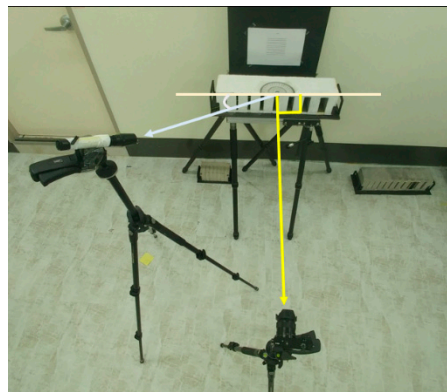
Figure B1. Test setup for analysis of lighting angle and intensity of cracks.
