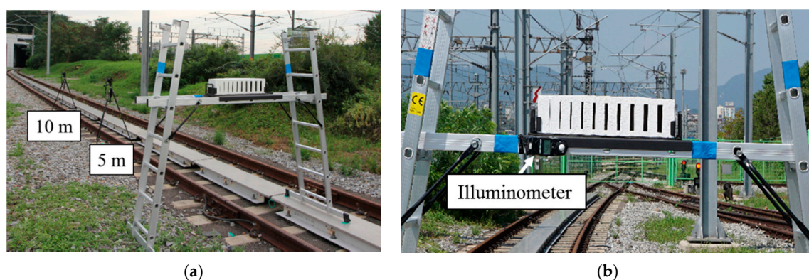
Figure 7. Image acquisition apparatus configuration: (a) Camera settings; (b) Illuminometer installation.
