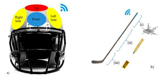
Figure 6. Instrumented smart helmet (a) and instrumented smart stick (b).
