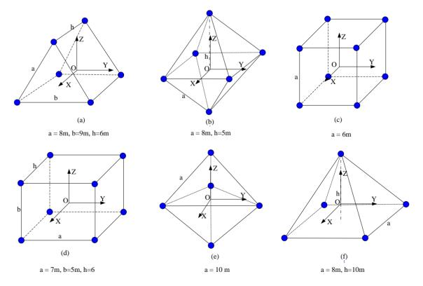
Figure 4. The geometric layouts of the ERS points. (a) Triangular prism layout; (b) Double rectangular pyramid layout; (c) Cube layout; (d) Cuboid layout; (e) Double triangular pyramid layout; (f) Rectangular pyramid layout.
