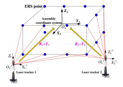
Figure 1. The measurement principle in large-scale aircraft assembly systems.
