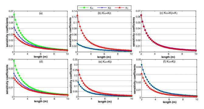
Figure 5. The sensitivity coefficients of rotation parameter errors versus volume size. (a) Sensitivity coefficients of layout a; (b) Sensitivity coefficients of layout b; (c) Sensitivity coefficients of layout c; (d) Sensitivity coefficients of layout d; (e) Sensitivity coefficients of layout e; (f) Sensitivity coefficients of layout f.
