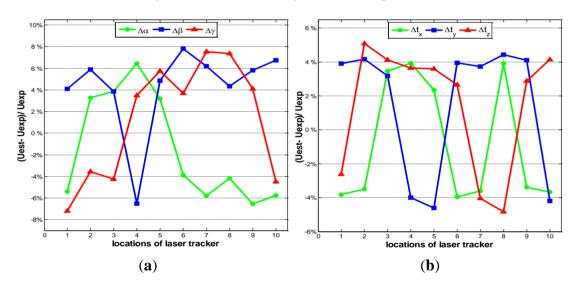
**Figure 3.** The relative estimation errors of the uncertainties of transformation parameter errors. (a) The estimation errors of the uncertainties of rotation parameter errors; (b) The estimation errors of the uncertainties of translation parameter errors.
