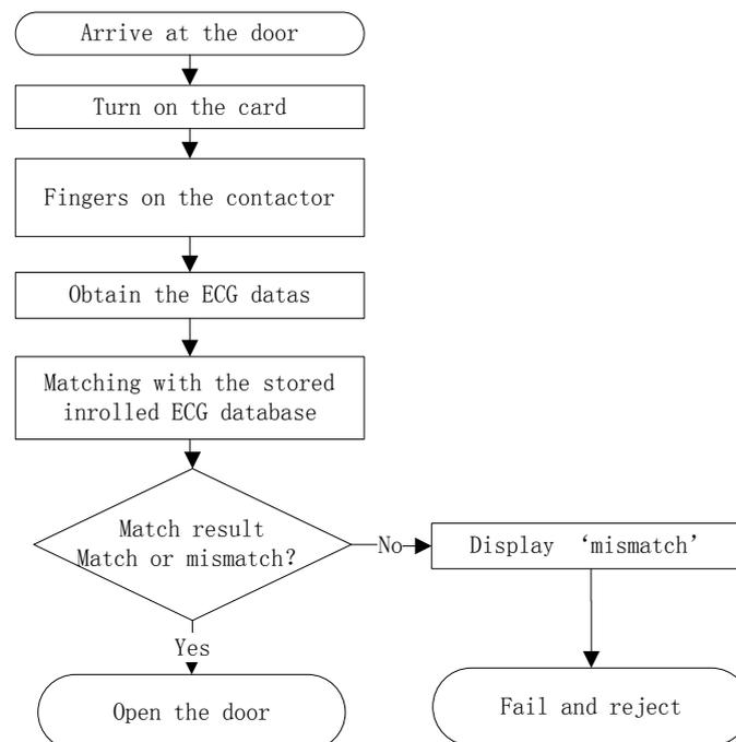
**Figure 5.** Flow chart of ECG verification processing.
