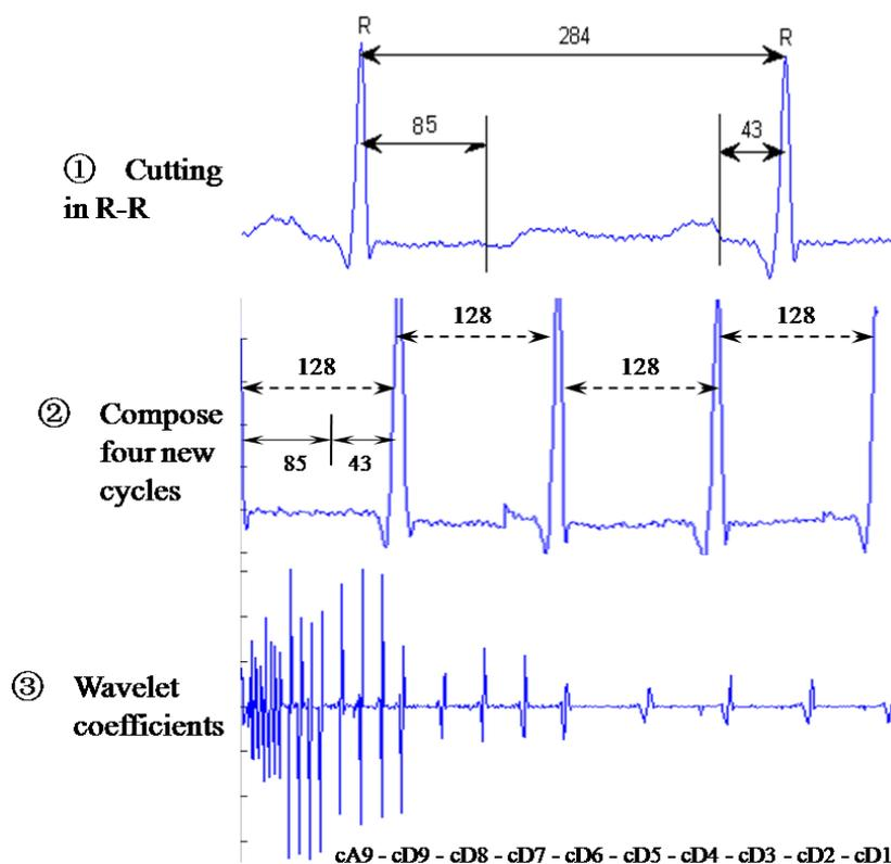
**Figure 10.** Procedure of the wavelet-based algorithm.
