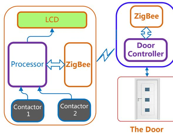
**Figure 4.** Door access control: Application of ECG sensor card.
