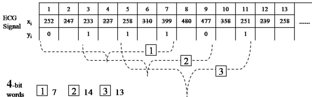
**Figure 8.** Process of the modified reduced binary pattern conversion.
