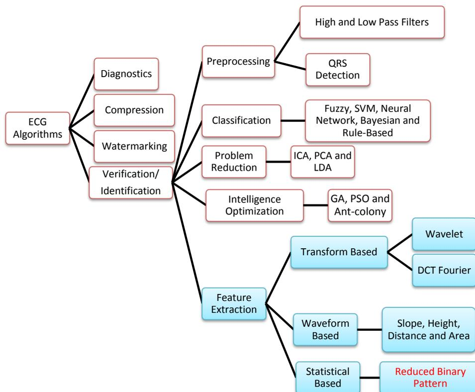
**Figure 1.** The classification of ECG algorithms.
