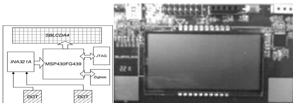
**Figure 3.** Architecture and hardware implementation of ECG sensor card.
