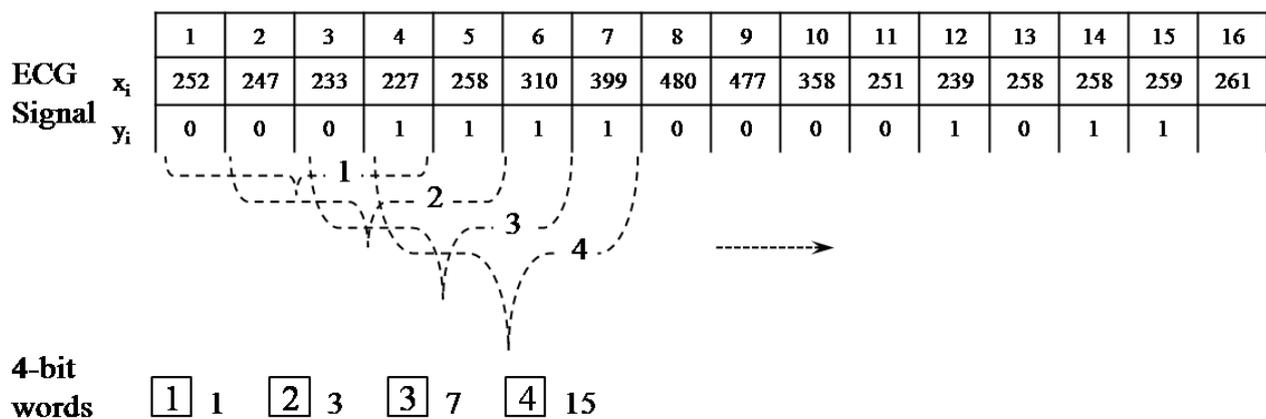
**Figure 6.** Process of the reduced binary pattern conversion.
