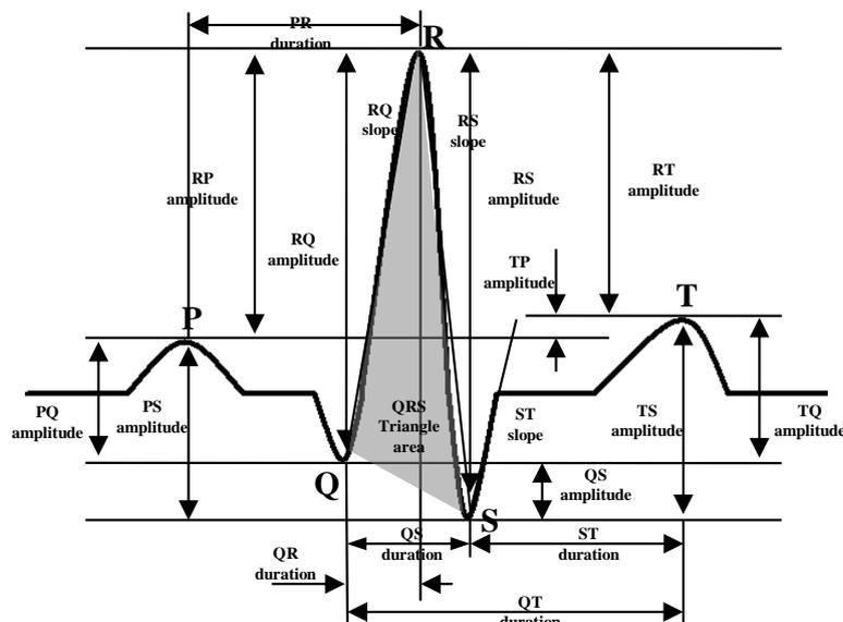
**Figure 9.** Waveform feature extraction for verification.
