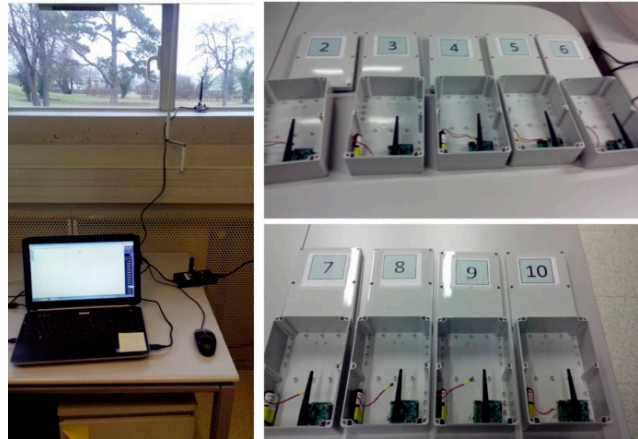
Figure 6. Testbed setup: sink node and nine IWoTCore Ext_MiLive nodes for outdoor environment experiments.
