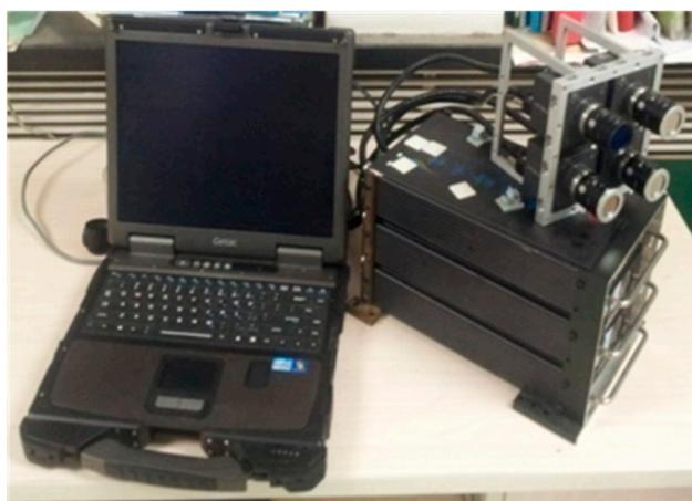
**Figure 1.** The four-camera multispectral mapping system.
