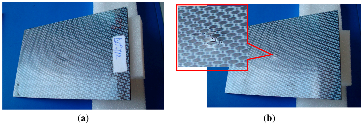
Figure 7. Sample impacted with 12 J energy: (a) front side; (b) back side—inset: breaking of fibers.
