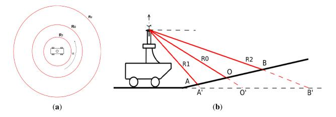
Figure 4. Radar beam model for flat, horizontal ground, up view (a); Uphill ground in view of the radar (b).
