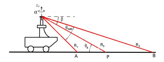
Figure 1. A vehicle equipped with a millimetre-wave (MMW) radar to perform terrain analysis.
