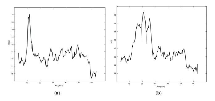
**Figure 7.** Examples of false positives: an obstacle would be erroneously labeled as ground considering only the SE (**a**); an obstacle in the vicinity of ground would be flagged as ground (**b**). Black: radar observation. Grey: RCGD ground echo model.
