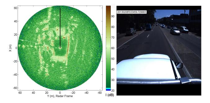
**Figure 2.** Example of radar image (**Left**). Note that the forward direction of the vehicle is marked by the black line. Front view of the vehicle (**Right**), as acquired by a co-located camera.
