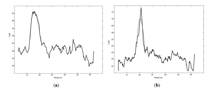
**Figure 6.** Example of good fit (SE = 94.0  $dB^2$ ) (**a**), and poor fit (SE = 913.1  $dB^2$ ) (**b**). Black: radar observation. Grey: Radar-Centric Ground Detection (RCGD) ground echo model.
