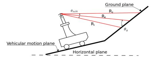
**Figure 5.** Radar-based ground detection in a general environment where motion plane and area under investigation do not coincide.
