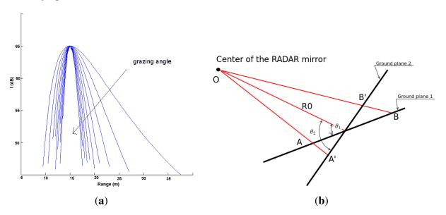
Figure 3. Change in the ground-echo model for increasing grazing angles, as indicated by the arrow in figure ( $R_0 = 15 m$ ,  $I_{R_0} = 65 dB$ ),  $\theta_g = 3-12^\circ$  (a); Change in the footprint and range-spread as a function of  $\theta_g$  while  $R_0$  is kept constant (b).
