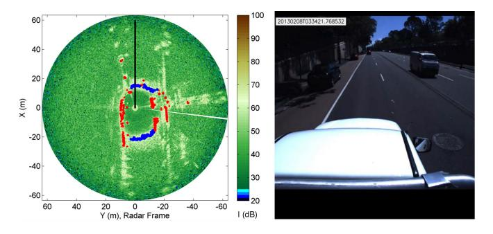
**Figure 10.** Classification results obtained from the RCGD method overlaid over the radar image (**Left**) in a typical urban environment (**Right**). Blue dot: Radar-labelled ground. Red dot: Radar-labeled obstacle.
