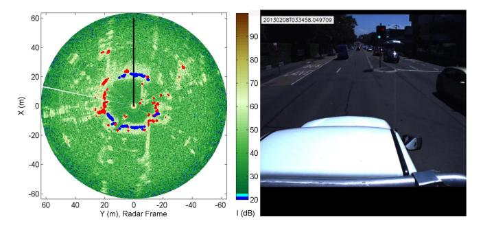
**Figure 11.** Output of the RCGD algorithm overlaid over the radar image (**Left**) in a cluttered urban environment (**Right**). Blue dot: Radar-labelled ground.
