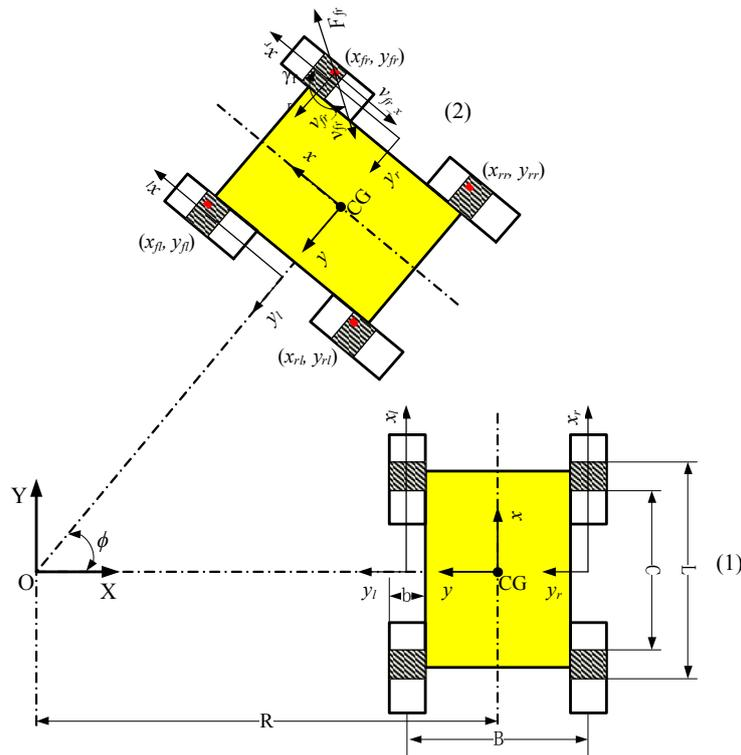
**Figure 4.** Motion of the skid-steering mobile robot wheel element on the lab surface (firm ground) from position (1) to (2).
