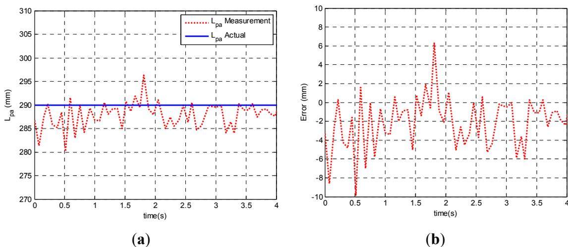
**Figure 10.** (a) A comparison of the measured width of the plate from the laser scanner and the actual value; (b) Error between measured width and actual one.
