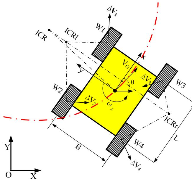
**Figure 1.** The kinematics schematic of skid-steering mobile robot.
