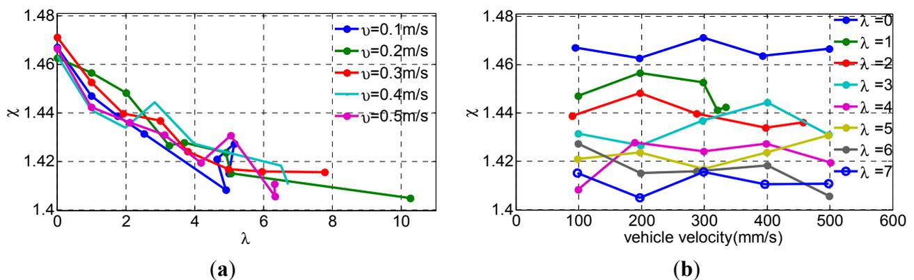
**Figure 12.** The calculated ICR coefficient  $\chi$  for various: (a) path curvatures with  $v = 0.1, 0.2, \dots, 0.5$  m/s ; and (b) robot speeds with  $v = 0.1, 0.2, \dots, 0.5$  m/s with  $\lambda = 0, 1, 2, \dots, 7$ .
