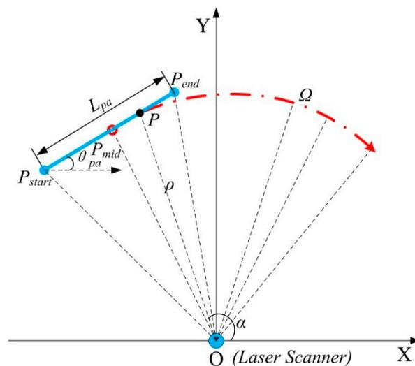
**Figure 8.** Position and heading measurement from the plate based on LMS400-1000 Laser Scanner for a real trajectory  $\Omega$  of the robot's center.
