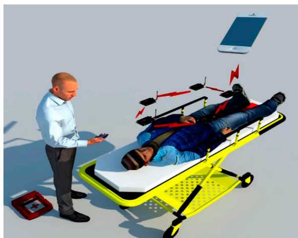
Figure 2. Wireless body sensor network communicating through a mobile phone.
