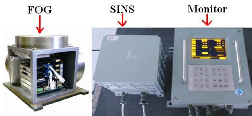
**Figure 5.** The FOG and FOG-based SINS.
