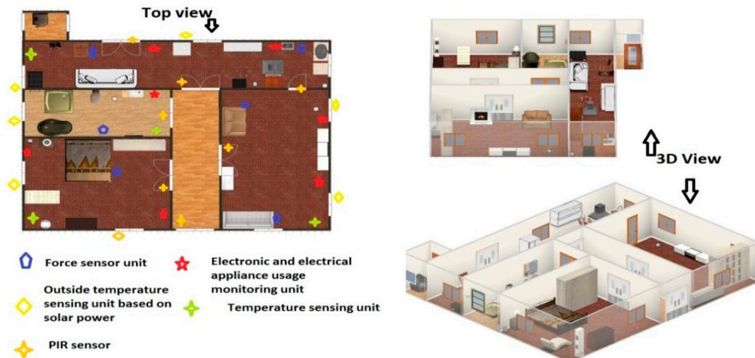
**Figure 2.** Layout structure of the house with sensor deployment and household objects.
