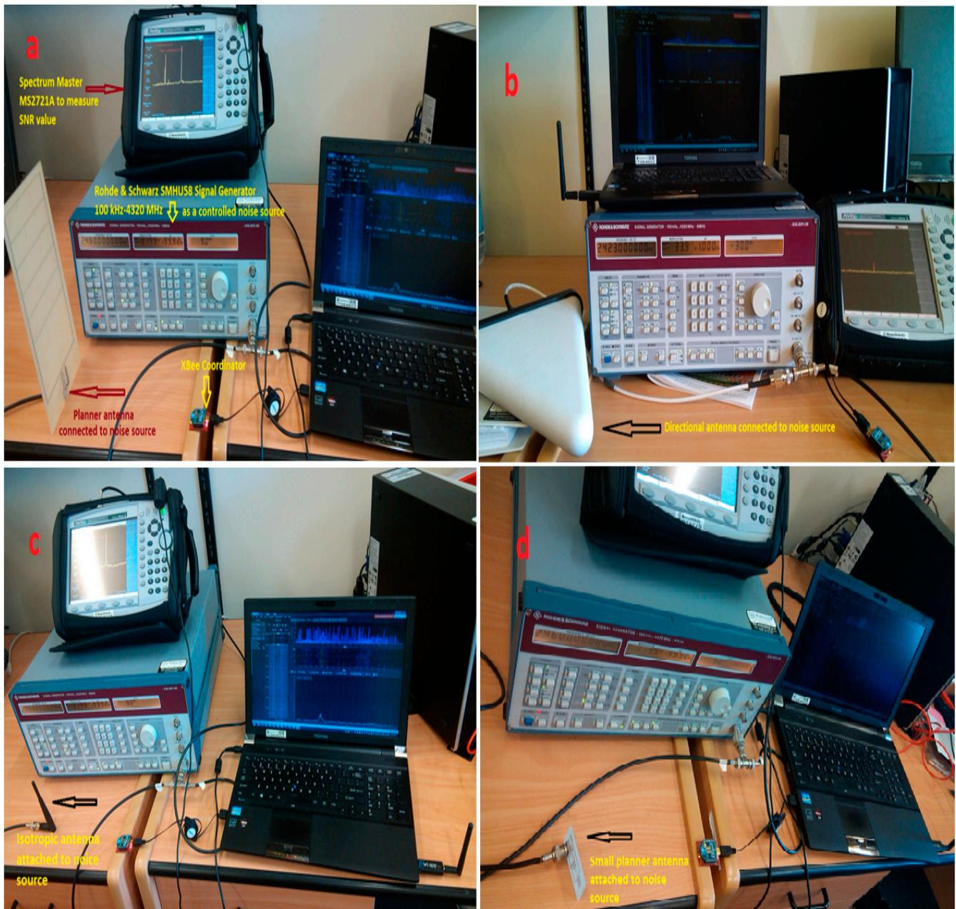
**Figure 18.** Controlled noise setup to investigate the interference characteristics of the smart building environment; (a) External noise generated by planner antenna; (b) External noise generated by directional antenna; (c) External noise generated by isotropic antenna and (d) External noise generated by small planner antenna.
