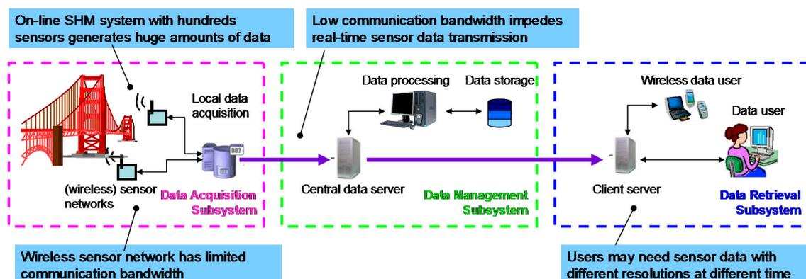
**Figure 1.** Schematics of an on-line structural health monitoring system and technical challenges.
