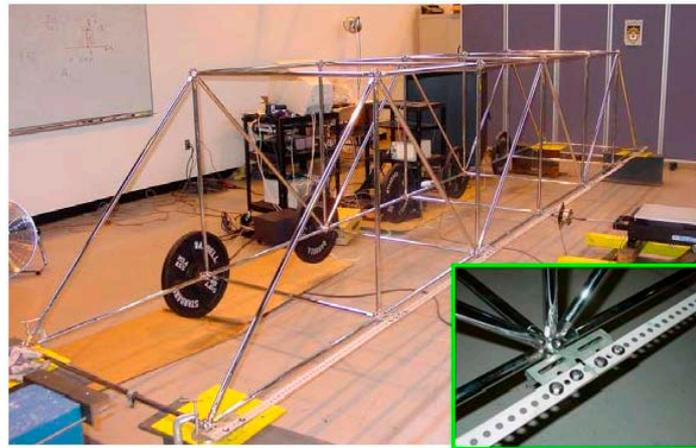
**Figure 2.** View of scaled steel bridge structure (inset shows the connection detail).
