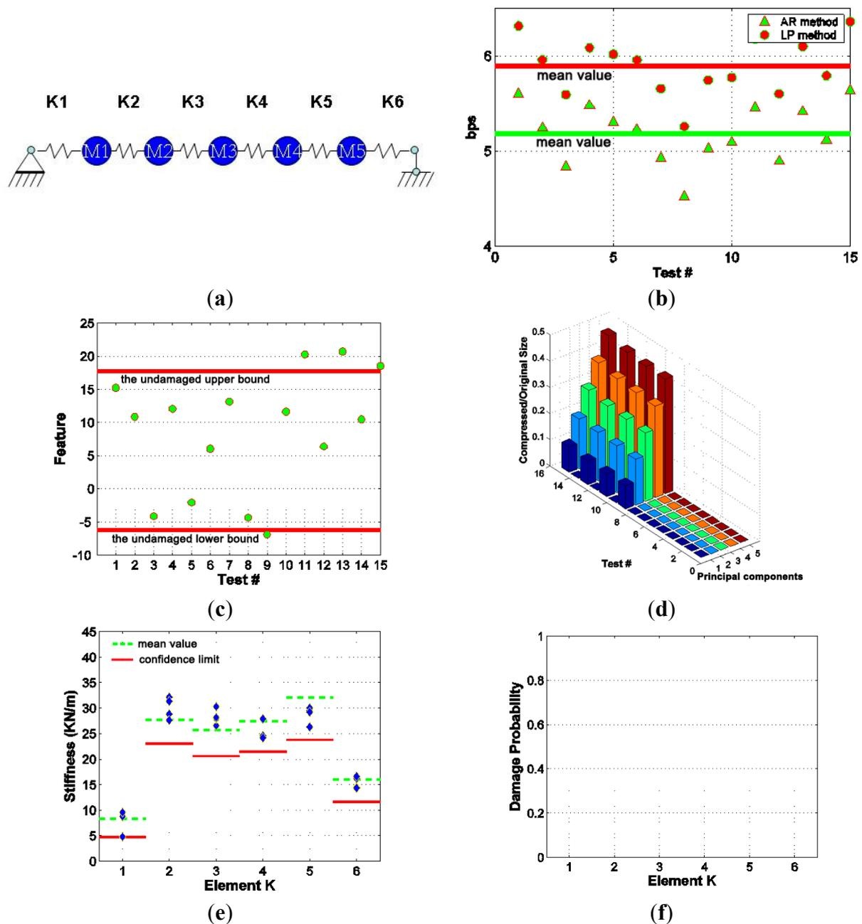
**Figure 8.** Performance of Integrated SHM system in Scenario #3 (a) Retrofitted structure (w/o damage); (b) Sensor data compression; (c) Feature monitoring; (d) Progressive data transmission; (e) Identified stiffness; (f) Statistical analysis of damage.
