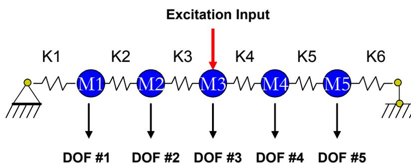
**Figure 3.** Idealized lumped-mass model for the steel bridge structure.
