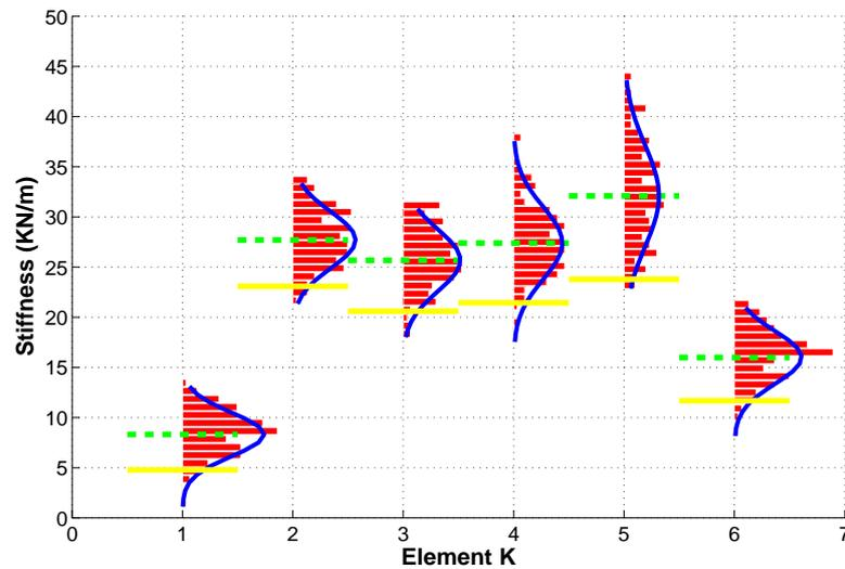
**Figure 5.** Control chart of identified stiffness coefficients.
