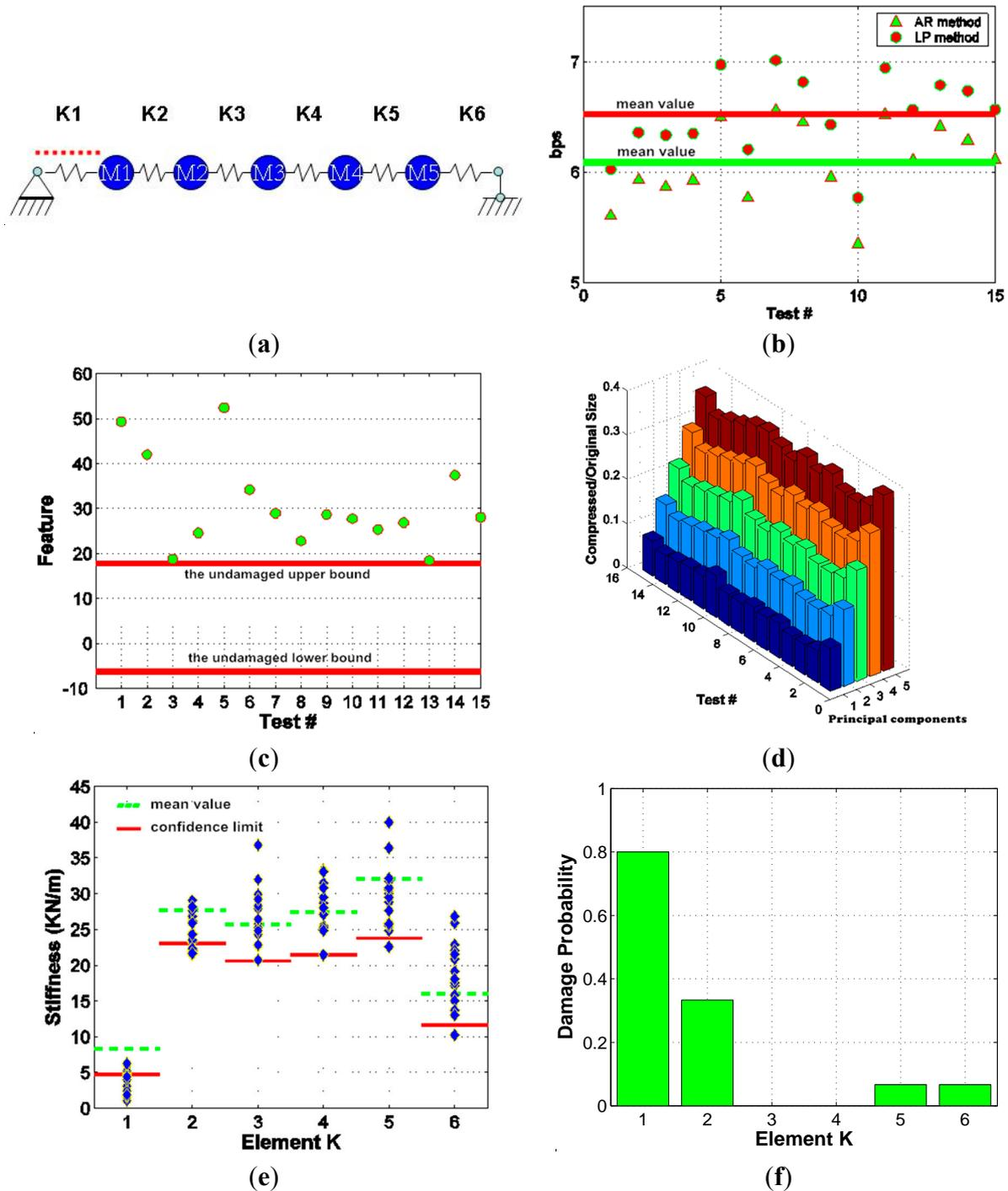
**Figure 6.** Performance of the Integrated SHM system in Scenario #1 (a) Damage at single location; (b) Sensor data compression; (c) Feature monitoring; (d) Progressive data transmission; (e) Identified stiffness; (f) Statistical analysis of damage.
