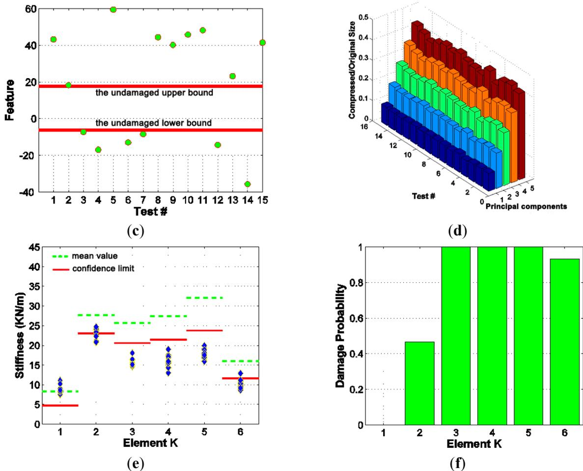
**Figure 7.** Performance of Integrated SHM system in Scenario #2 (a) Damage at multiple locations; (b) Sensor data compression; (c) Feature monitoring; (d) Progressive data transmission; (e) Identified stiffness; (f) Statistical analysis of damage.
