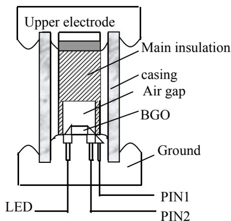
**Figure 3.** Structural diagram of a sensor.
