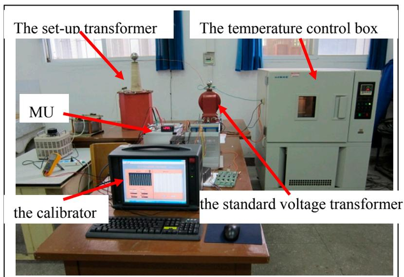
**Figure 5.** The Temperature Test Photo of OEFS.
