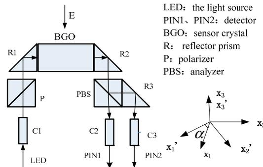
**Figure 2.** The principle of OEFS.
