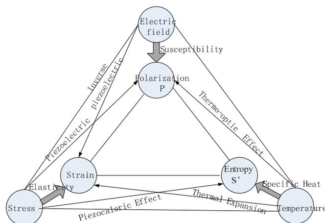
**Figure 1.** The relationship between various parameters of a crystal system.
