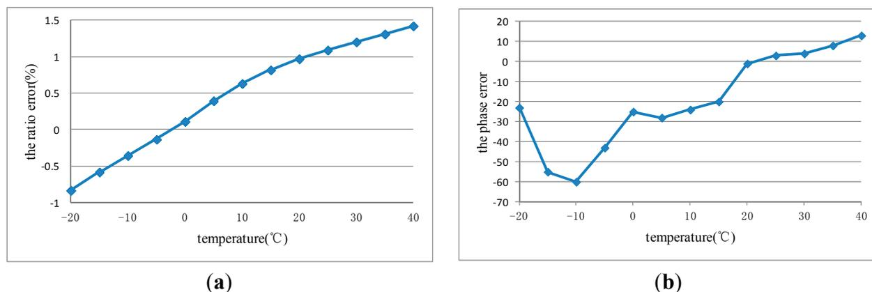
**Figure 7.** (a) The Ratio Error Curve with Temperature; (b) The Phase Error Curve with Temperature.
