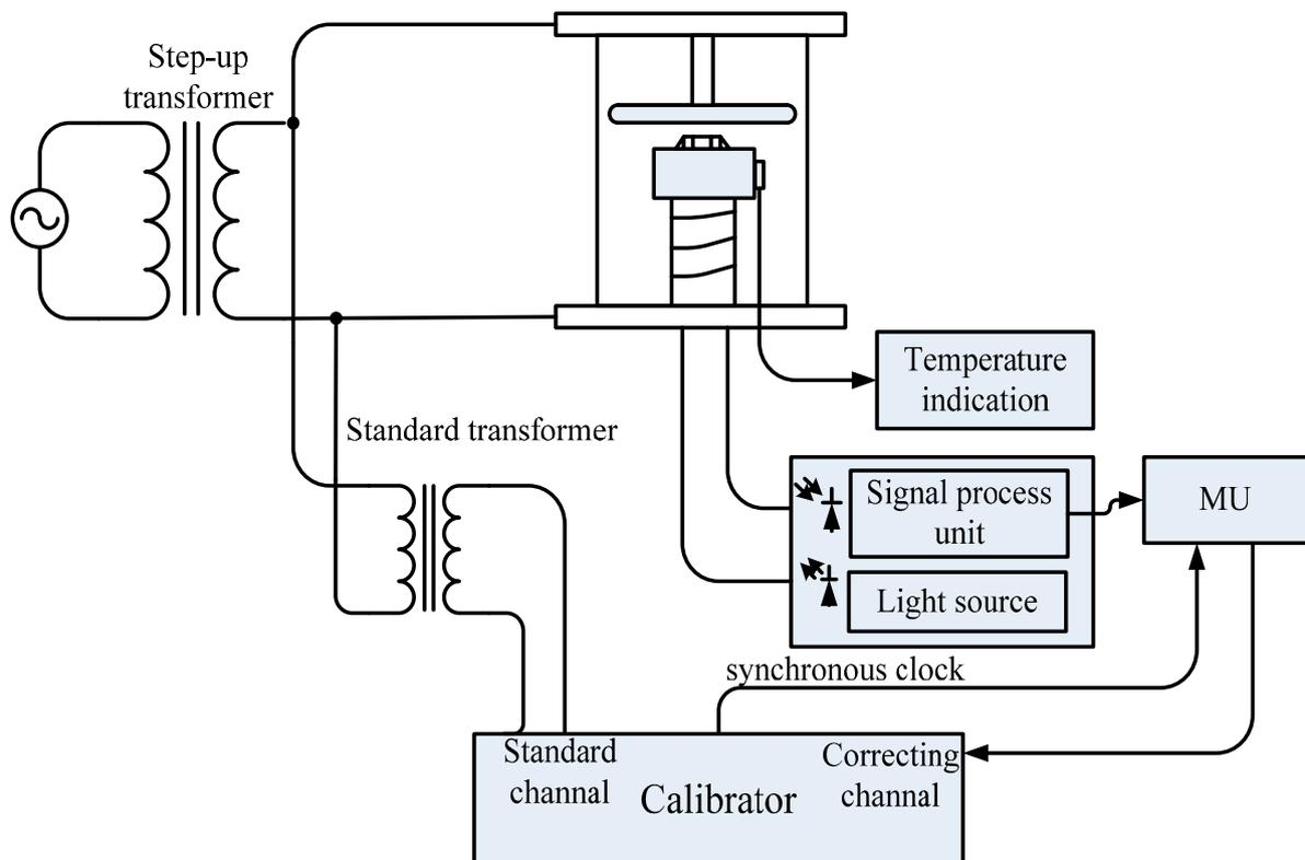
**Figure 4.** OEFS Tests Schematic Diagram.
