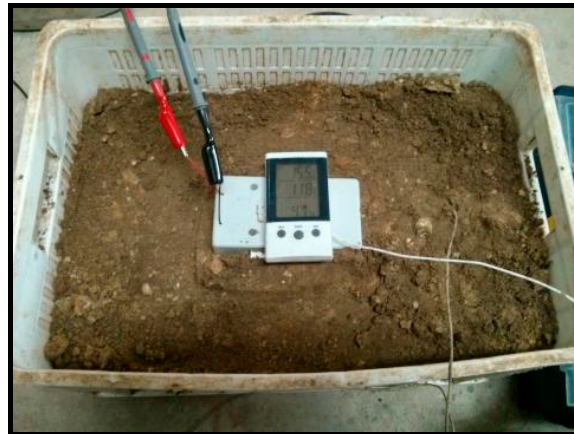
Figure 10. Peltier cell installed inside a plastic case and buried in the sand.
