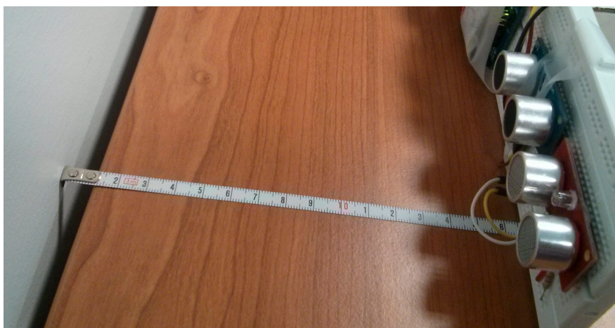
Figure 5. Short distance test of the ultrasonic distance sensors.
