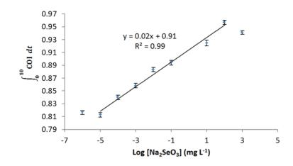
**Figure 7.** Dynamic range of *E. coli* roGFP2 oxidative stress biosensor towards the exposure of Na<sub>2</sub>SeO<sub>3</sub> (1 ng L<sup>-1</sup>–1000 mg L<sup>-1</sup>).  $\int_0^{10}$  COI *dt* indicates the total COI response of biosensor in 10 min. Error bars indicate the values of standard deviation (*n* = 8). The roGFP2-expressing *E. coli* cells were immobilized in 1.8% (w/v) KC at 4.5 × 10<sup>8</sup> cfu mL<sup>-1</sup>.
