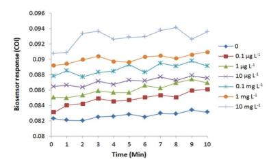
**Figure 4.** Cellular oxidation profile of *E. coli* roGFP2 oxidative stress biosensor exposed to NaAsO<sub>3</sub> (0.1  $\mu$ g L<sup>-1</sup>–100 mg L<sup>-1</sup>). A typical result out of 4 replicates is shown. The roGFP2-expressing *E. coli* cells were immobilized in 1.8% (w/v) KC at 4.5 × 10<sup>8</sup> cfu mL<sup>-1</sup>.
