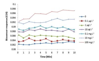
**Figure 6.** Cellular oxidation profile of *E. coli* roGFP2 oxidative stress biosensor exposed to Na<sub>2</sub>SeO<sub>3</sub> (0.1  $\mu$ g L<sup>-1</sup>–100 mg L<sup>-1</sup>). A typical result out of 4 replicates is shown. The roGFP2-expressing *E. coli* cells were immobilized in 1.8% (w/v) KC at 4.5 × 10<sup>8</sup> cfu mL<sup>-1</sup>.
