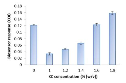
**Figure 2.** Responses of *E. coli* roGFP2 oxidative stress biosensors embed in several concentrations of KC. The cell density of *E. coli* roGFP2 was fixed at  $4.5 \times 10^8$  cfu mL<sup>-1</sup>. The biosensor was exposed to 1 mg L<sup>-1</sup> menadione. Cells suspended in the HEPES buffer act as control (0%). Error bars indicate standard deviation (*n* = 8).
