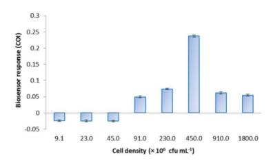
**Figure 3.** Responses of *E. coli* roGFP2 oxidative stress biosensors prepared with various cell densities immobilized in 1.8% (w/v) KC to 1 mg L<sup>-1</sup> menadione exposure. Error bars indicate the values of standard deviation (n = 8). Negative COI values indicate apparent reduction of the biosensors.
