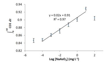
**Figure 5.** Dynamic range of *E. coli* roGFP2 oxidative stress biosensor towards NaAsO<sub>3</sub> exposure (10 ng L<sup>-1</sup>–100 mg L<sup>-1</sup>).  $\int_0^{10}$  COI *dt* indicates the total COI response of biosensor in 10 min. Error bars indicate the values of standard deviation (*n* = 8). Solid line and inset equation indicate linear regression of the plots. The roGFP2-expressing *E. coli* cells were immobilized in 1.8% (w/v) KC at 4.5 × 10<sup>8</sup> cfu mL<sup>-1</sup>.
