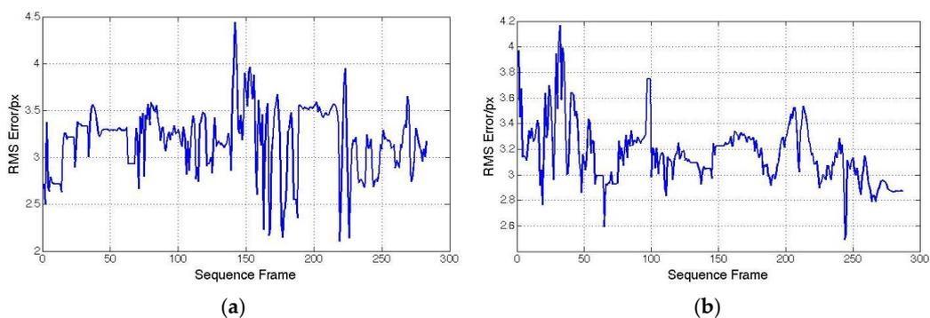
**Figure 10.** Re-projection error of hybrid tracking method. (a) Rotate along Y-axis; (b) Move backwards and forwards.
