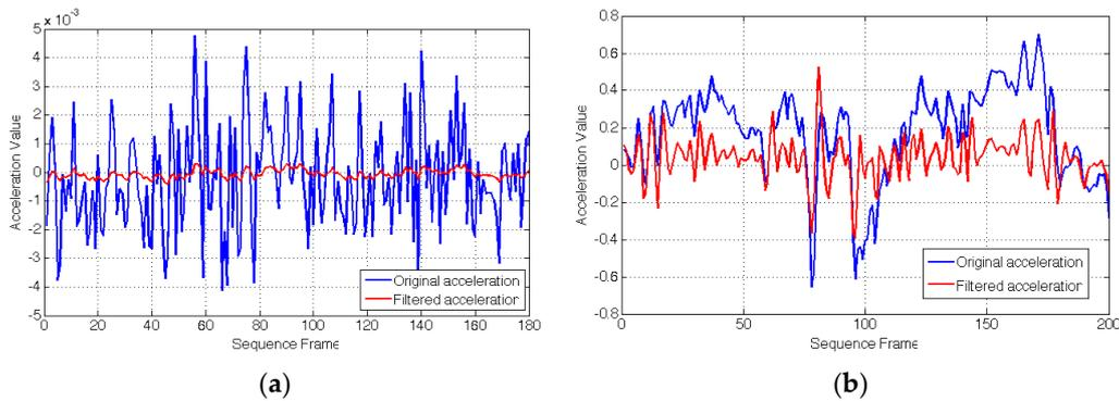
**Figure 9.** Effect of de-noising. (a) Static; (b) Random moving.
