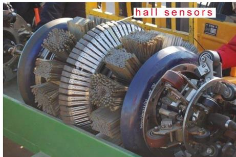
**Figure 10.** Photo of the magnetic pig with the Hall sensors.
