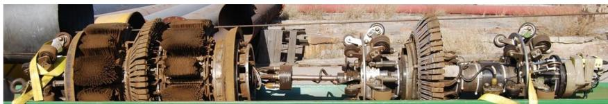
**Figure 1.** A MFL tool, comprising three main sections: a drive section at the front of the tool, a central magnetizer section and a data logger situated towards the rear of the tool.
