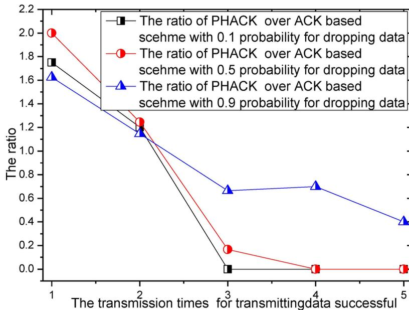
Figure 17. The ratio of PHACK and the ACK-based scheme with different rates for the dropping of data.
