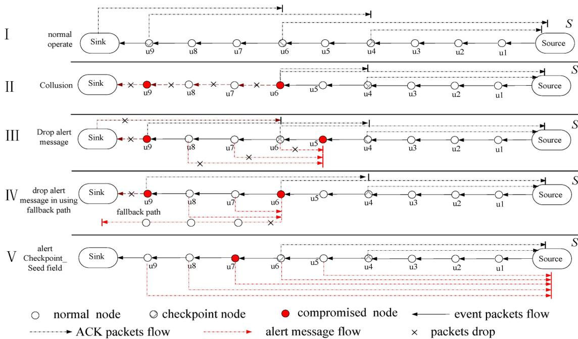
Figure 1. Overview of acknowledgment-based selective forwarding attack detection.
