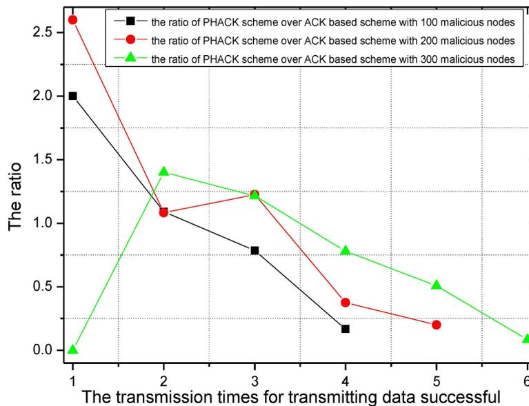
Figure 13. The ratio of transmission times for successful data transmission of PHACK over that of the ACK-based scheme.
