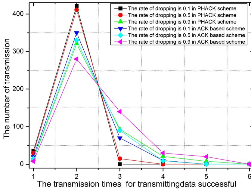
Figure 16. The number of successful data transmissions in the PHACK scheme with different rates for the dropping of data.
