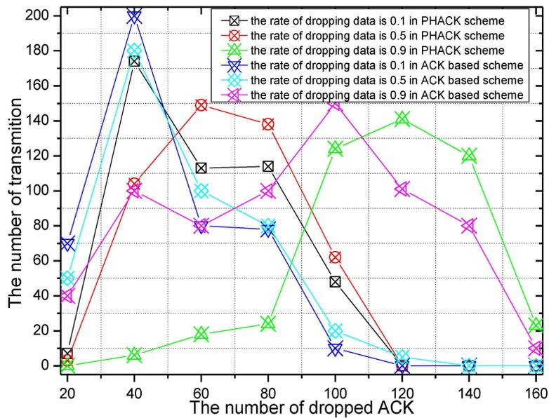
Figure 18. The number of dropped ACKs with different rates for dropping data.
