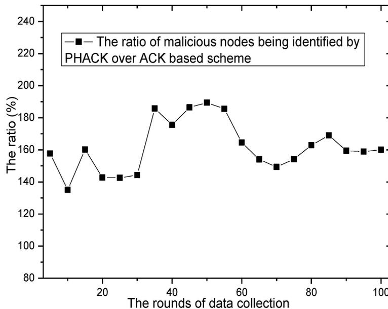
Figure 21. The ratio of malicious nodes being identified by PHACK over the ACK-based scheme.
