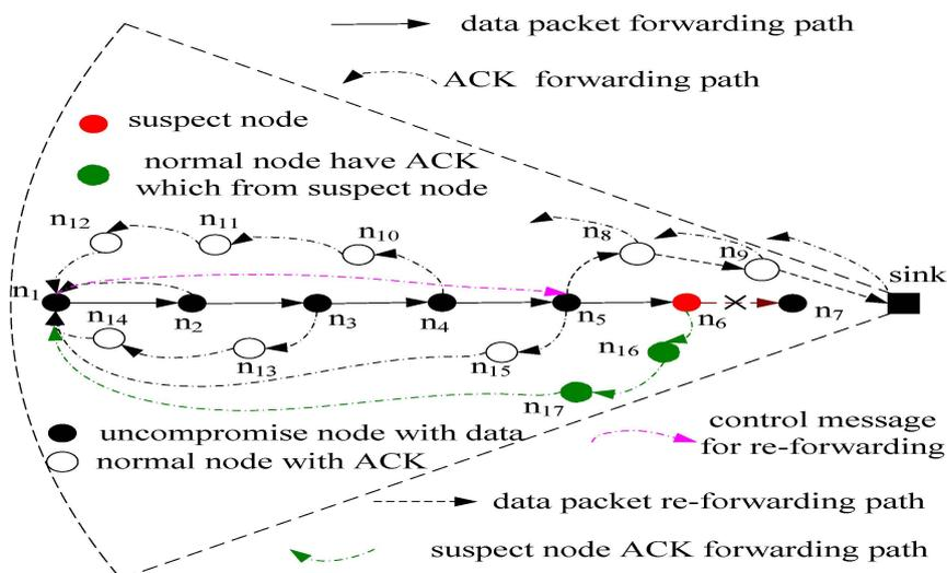
Figure 2. Illustration of the PHACK scheme.
