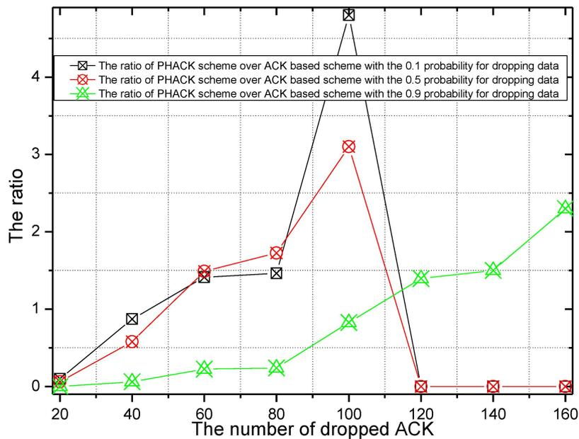
Figure 19. The ACK dropping ratio of PHACK over the ACK-based scheme.
