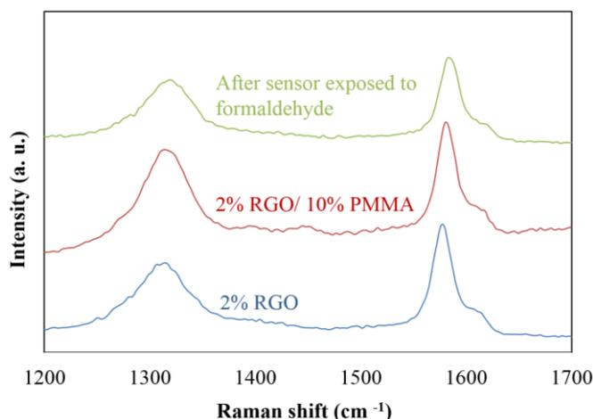
**Figure 5.** Raman spectroscopy ( $E_L = 1.59$  eV and  $\lambda_L = 780$  nm) of the RGO-based sensing materials.
