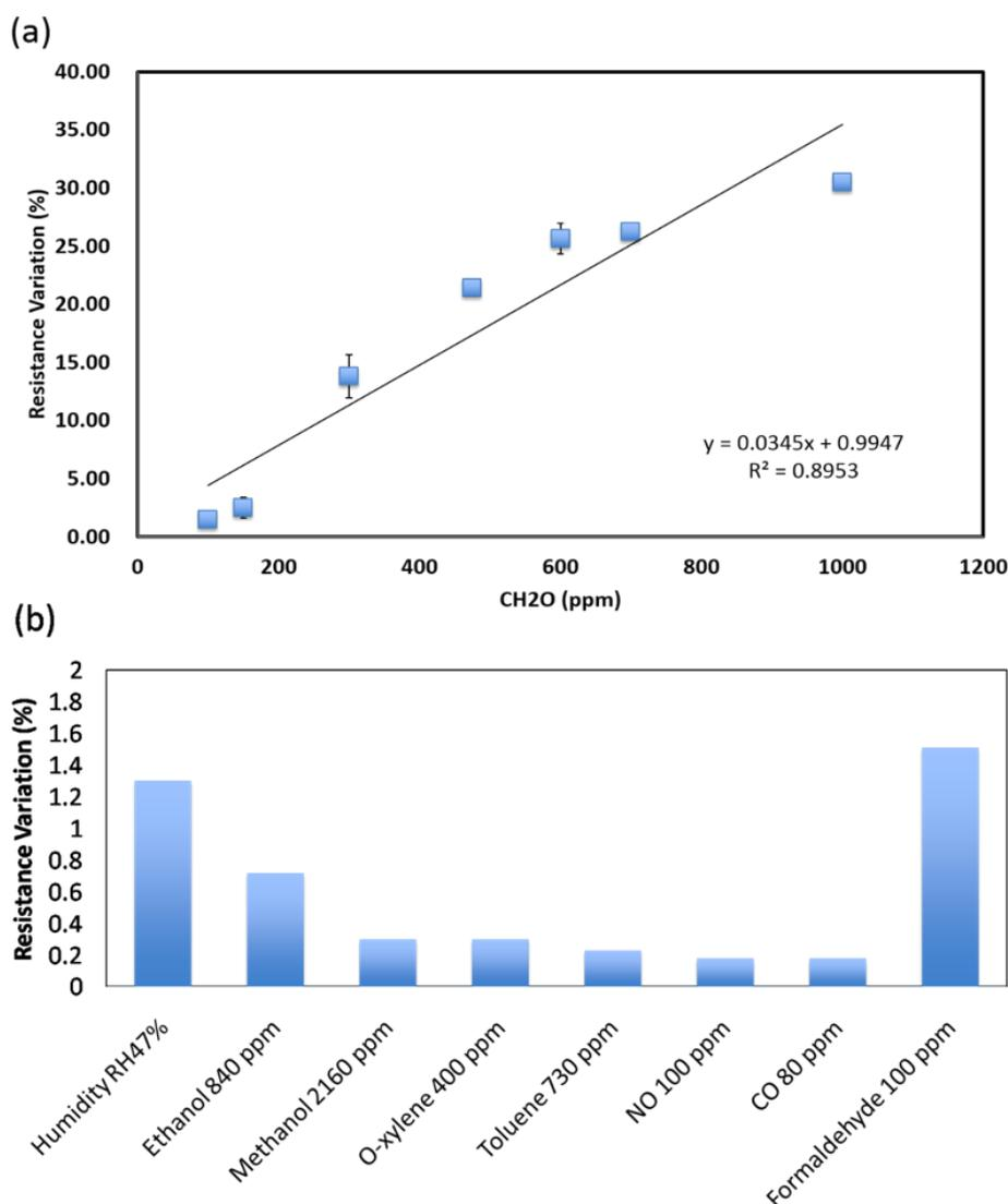
**Figure 4.** The characteristics of 2% RGO/ 10% PMMA sensing material operated at room temperature for: (a) formaldehyde sensitivity and (b) selectivity.
