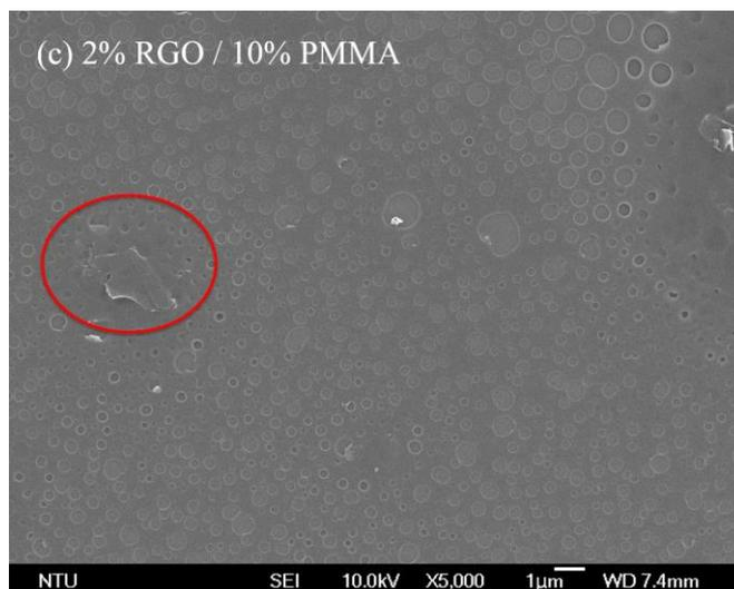
**Figure 1.** SEM pictures of different RGO/PMMA sensing film compositions: (a) 2% RGO, (b) 2% RGO/5% PMMA, and (c) 2% RGO/10% PMMA composite. The red circles indicate the graphene sheets.
