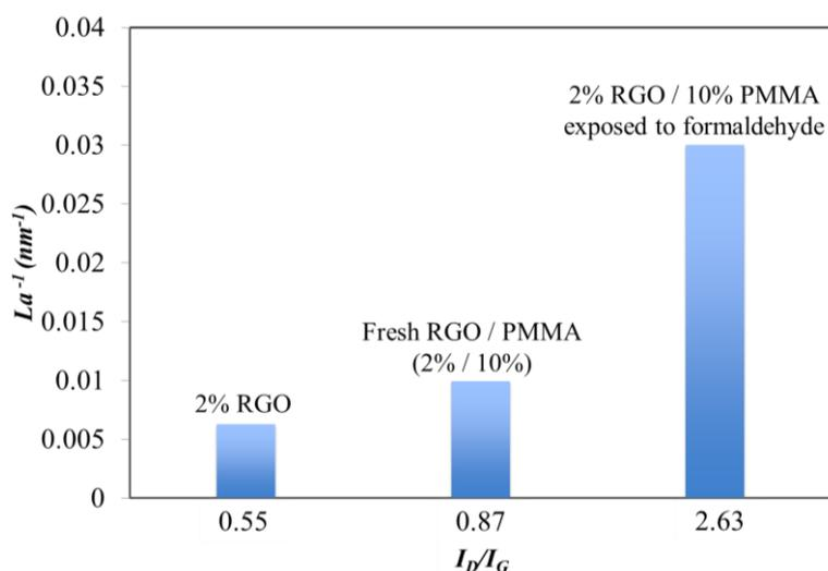
**Figure 6.** Dependency of the  $I_D/I_G$  ratio and the inverse values of crystallite diameter for RGO-based sensing films.
