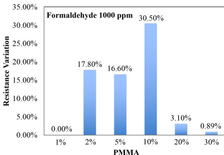
**Figure 3.** The formaldehyde sensing result of different PMMA blending concentrations with 2% RGO
