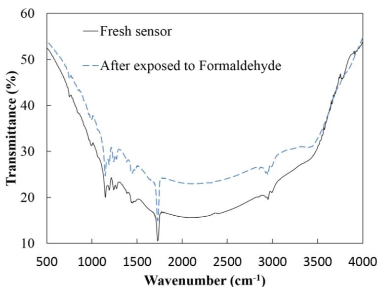
**Figure 2.** FTIR analysis for fresh RGO/PMMA based sensor (black line) and after sensor exposed to formaldehyde (dashed line).
