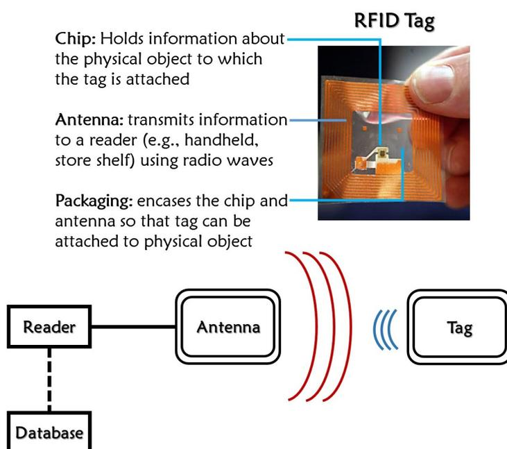
**Figure 1.** Wireless sensor scenario (radio frequency identification (RFID) system).
