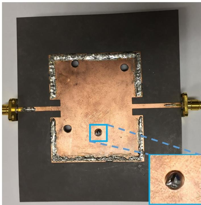
**Figure 5.** Photograph of the fabricated prototype at state 2 (0001). The magnified inset shows the liquid metal (LM)-filled channel after injecting eutectic gallium indium (EGaIn) into the channel 4.
