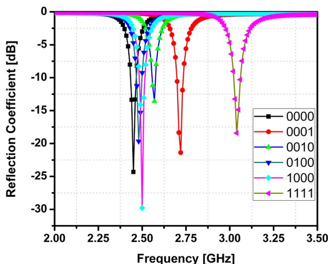
**Figure 3.** Simulated reflection coefficients of the proposed SIW resonator.
