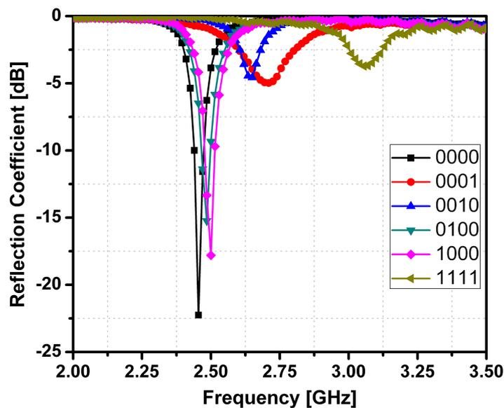
**Figure 6.** Measured Reflection Coefficients of Proposed SIW resonator.
