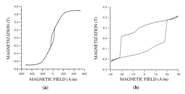
Figure 11. Bistable samples: (a) hysteresis loop; (b) Minor loop.
