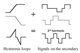
Figure 9. Signal of each core applying an external field.
