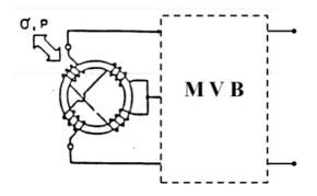
Figure 4. Sensor used as anti-aircraft position system with a multivibrator bridge (MVB).
