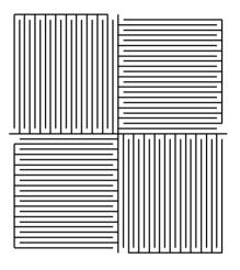
Figure 13. Resistance bridge with conductive bands forming a 90 ° angle between them.
