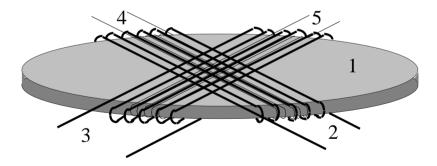
**Figure 10.** Schematic view of two-axis sensor unit. 1: Amorphous disc. 2/3: Orthogonal primary coils. 4/5: Orthogonal pick-up coils [21].
