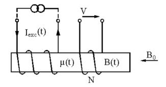
Figure 7. Magnetometer sensor with single core [20].
