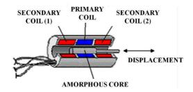
Figure 14. LVDT experimental set-up.
