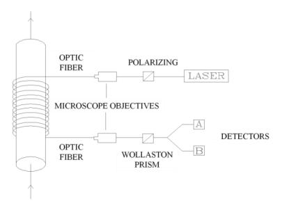
Figure 5. Current sensor based on material length variation with magnetic direction.
