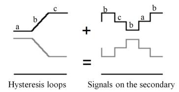
Figure 8. Signal of each core without external field applied.
