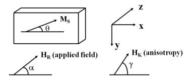
Figure 12. Magnetization, applied magnetic field and anisotropy direction.
