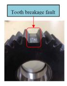
Figure 25. The photograph of tooth breakage fault in planet gear.
