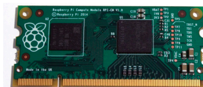
Figure 7. The RPI Compute Model; 67.6 × 30 mm board as DDR2 SODIMM (Source: Raspberry PI website).
