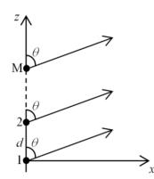
The PA total far field ( $E_T$ ) is equal to the field of an element positioned at the reference point ( $E_{el}$ ) multiplied by the array field, or array factor, AF, as summarized in Equation (1) [7]. This process is called multiplication of radiation patterns and can be extended to PAs of several elements [7,8]. In general, AF depends only on the geometry and excitation of PA, which eases projects designed to isotropic elements and then extrapolated to any type of element.
