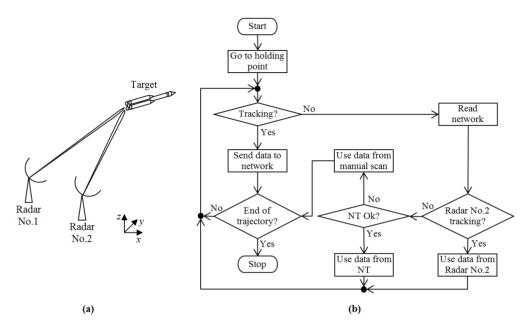
Figure 3. (a) Rocket Tracking System (RTS) with two radar sensors. (b) Flowchart of operation of the Radar No.1.
