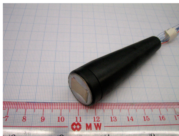
Figure 19. Photography of as-fabricated cylindrically shaped ultrasonic linear array.
