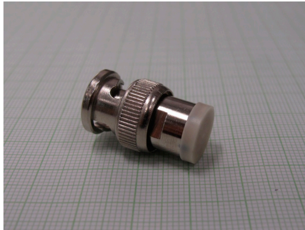
Figure 13. Photograph of the 1-3 composite single-element ultrasonic transducer (with permission from [79]).
