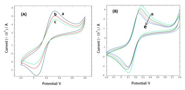
At the aptamer modified electrode, the electrochemical reaction of the redox probe is prevented and an increase in the peak-to-peak separation and a decrease in the peak current is observed. The
