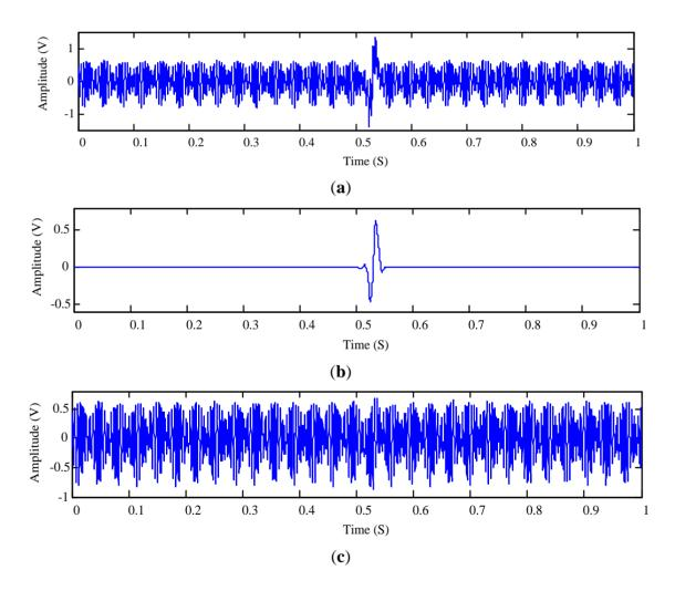
The RMSDK\_SSR value of the residue signal shown in Figure 14c is 0.030438 which is lower than 0.031020 obtained by the joint time-invariance wavelet transform and kurtosis approach. This result again indicates that the proposed approach outperforms the reference approach in terms of the quality of the extracted particle signature.
