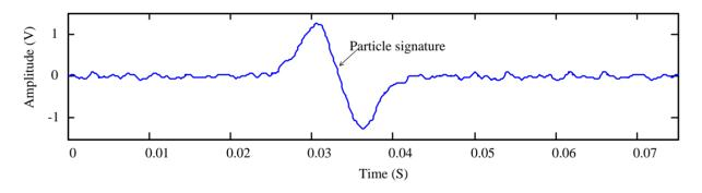
As is introduced in Section 1 and shown in Figure 2, the metallic particle signature is similar to a  $2\pi$  sinusoidal waveform that can be simulated by:
