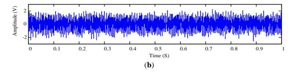
For comparison, we also employ the joint time-invariance wavelet transform and kurtosis approach [17] to process the same signal s(t). The decomposition depth used in the reference approach is calculated using Equation (16) as L = 10. With the wavelet-based approach from the reference, the extracted particle signature and the residue signal are obtained and displayed in Figure 13a,b, respectively.
