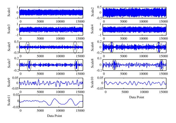
**Figure 5.** Wavelet coefficient shrinkages for all scales. For convenience, the profile coefficients of the scale 10 are marked as "scale 11". At each scale, coefficients related to particle signatures are highlighted using circles.
