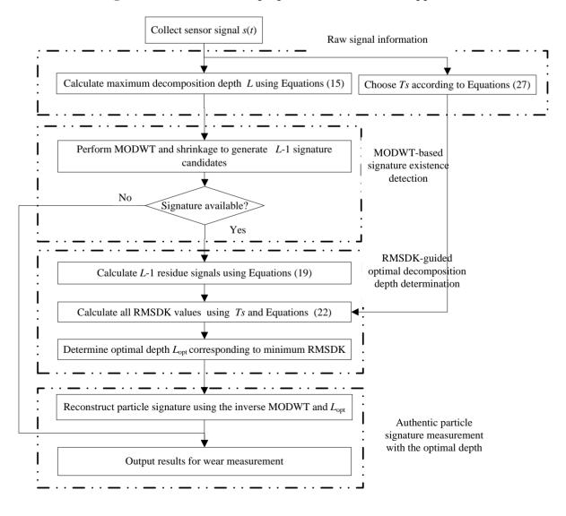
Figure 7. Flowchart of the proposed MODWT-ODD approach.
