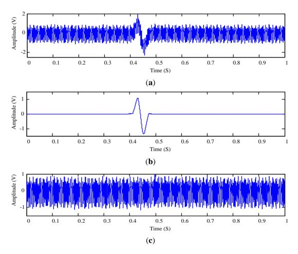
Through comparing three experiments under different SNRs, one can see that both the proposed and the reference wavelet-based approaches are able to detect the wear particle existences for the oil debris sensors. However, the proposed method is more effective in maintaining the integrity of the measured signature due to the introduction of the optimal decomposition depth  $L_{opt}$ .
