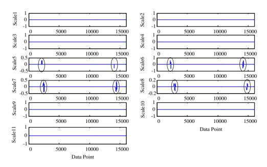
The shrunk coefficients are subsequently used to reconstruct the signal which more clearly displays the particle signature  $s_1(t)$  (Figure 6).
