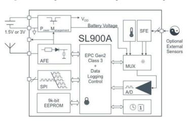
Figure 3. Temperature sensor chip structure diagram.
