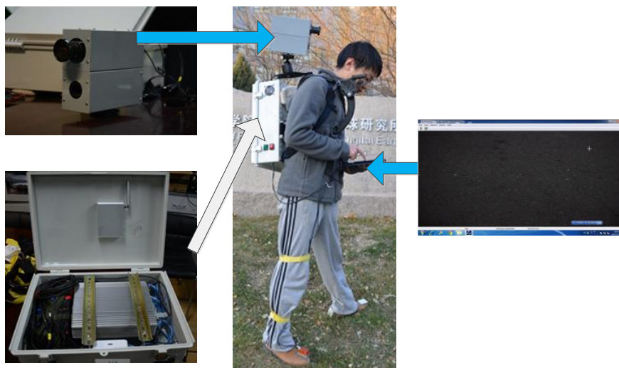
Figure 1. The hardware scheme for the astronaut navigation system.
