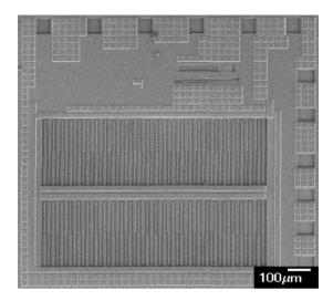
Figure 7. SEM images of the integrated humidity sensor after the wet etching.
