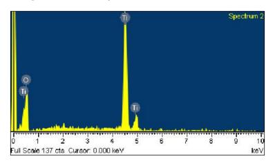
Figure 5. EDS analysis of the titanium dioxide film.
