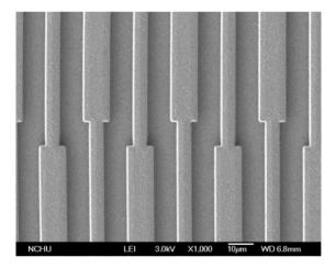
Figure 9. Optical image of the integrated humidity sensor after the post-process.
