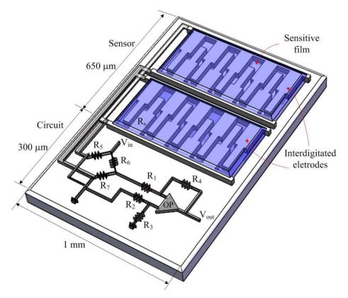
As shown in Figure 1, the integrated microsensor contains a readout circuit [24] to convert the resistance variation of the humidity sensor into the output voltage, where *OP* represents the operational amplifier,  $V_{in}$  is the input voltage of the circuit;  $V_{out}$  is the output voltage of the circuit;  $R_s$  is the resistance of the humidity sensor;  $R_1$ – $R_7$  are the resistances of the circuit.
