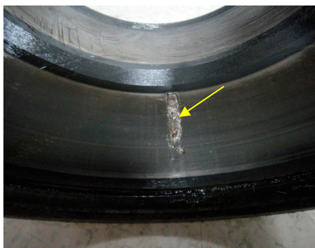
Figure 20. Outer-race of the dismantled bearing.
