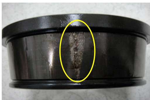
Figure 25. Inner-race of the dismantled bearing.
