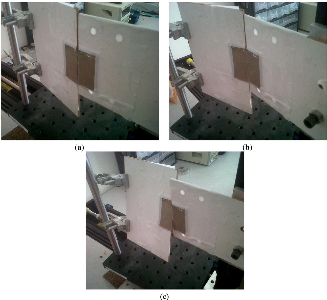
**Figure 6.** Shifting frequency of the metamaterial-based sensor *versus* displacement using the data experimentally obtained for possible misalignments: (a) inward bending of the NSRR parts, given for the angles of 5°, 10° and 15°; (b) outward bending of the NSRR parts, given for the angles of 5°, 10° and 15°; (c) twisting of the NSRR parts, given for the angles of 10°, 20° and 30°.
