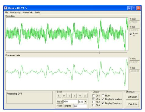
**Figure 6.** The effects of a single shot fast spin echo sequence gradient burst on the fECG trace (upper plot). The effects of a bandpass FIR filter are shown in the lower trace. The effects of the gradient pulses are largely removed from the trace but the phase of the ECG signal is temporarily altered.
