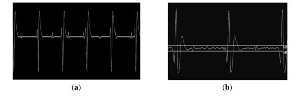
**Figure 4.** A FIESTA sequence with TR = 3.3 ms, TR = 1.4 ms, NEX = 1, in-plane spatial resolution =  $1 \times 1 \text{ mm}$ , SLT = 5 mm acquired with the cardiac gating signal from the simulated fetal ECG at 123 beats per minute acquired over the 6 m MR compatible leads. The images show no artifacts from the leads or electrodes.
