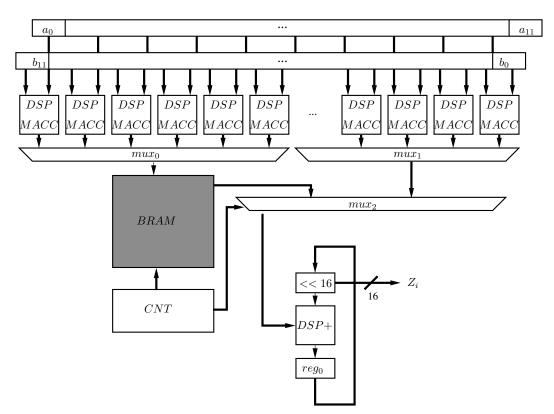
Since all the partial products are computed in parallel and are being added after the first partial product is generated ( $M_0$ ), the number of cycles for computing a multiplication is 23+1 (delay MACC) +1 (DSP addition) = 25 cycles.
