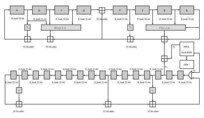
The message scheduler is initialized with the padded message at the beginning of the hash computation, whereas the main pipeline registers (**a**–**h**) are initialized with eight predefined words of 32 bits defined by the standard. The hash function involves the use of six logic functions (Ch, Maj,  $\Sigma_0$ ,  $\Sigma_1$ ,  $\sigma_0$  and  $\sigma_1$ ) defined in [18].
