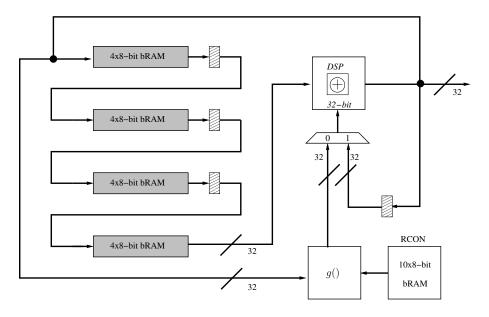
Since the CCM mode only requires the encryption part of AES, it can be implemented with two extra XOR gates of 32 bits (Figure 1). One is for the CBC operation and the beginning of the encryption. The other XOR gate is placed at the end for the XORing operation with the output of AES-CTR. Finally,
