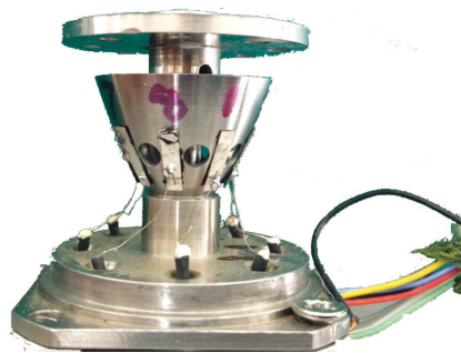
Figure 16. Prototypal bell-shaped resonator.
